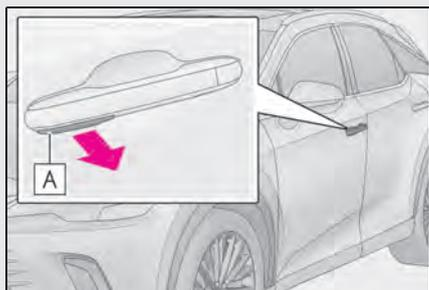
Pull the manual release handle **A** to open the door.
