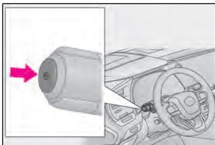
Press the Adaptive High-beam System switch.
