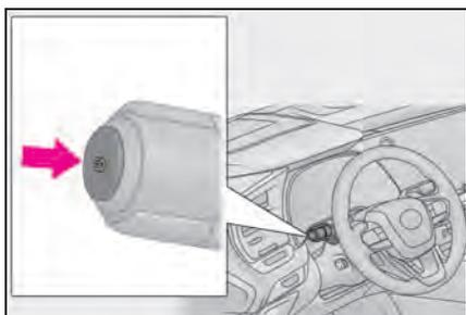
Press the Automatic High Beam switch.
