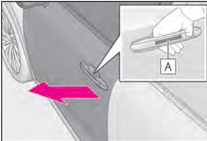
Press the door opener switch **A** of the door handle to open the door.
