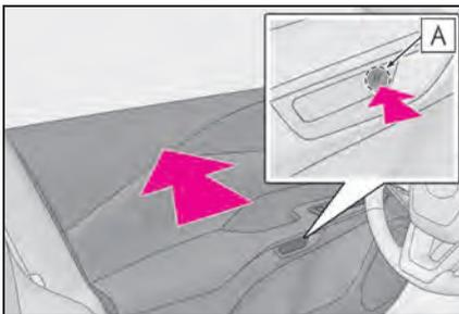
Press the front side of the door opener switch **A** to open the door.
