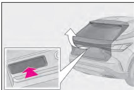
When the power back door is unlocked: Press the back door opener switch.
