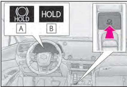
Turns the brake hold system on
