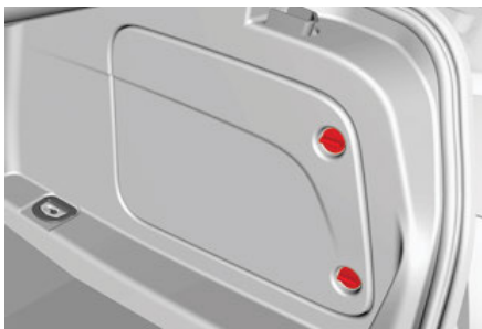
Battery Access Panel
