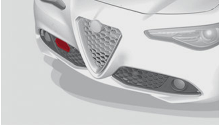
Front Fascia/Bumper Radar Location
