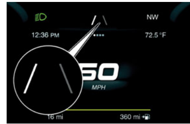
Left Lane Marking Detected
