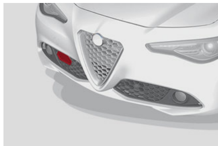
Front Bumper Radar Location
