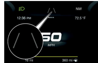
Lane Markings Not Detected
