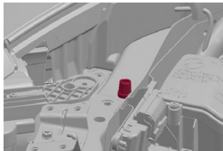
Remote Negative (-) Post Location
