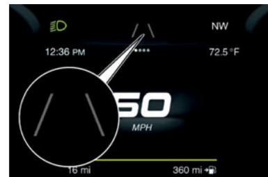
Lane Markings Not Detected
