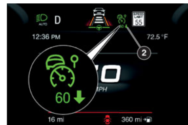
2 — Suggested Speed Lower Than Current Speed
