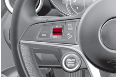
SET Switch Location
