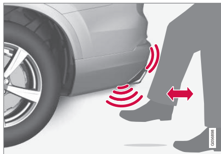
Kicking motion within the detector's activation area.
