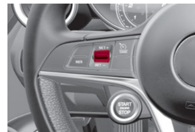
SET Switch Location
