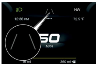
Lane Markings Not Detected
