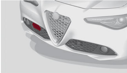
Front Fascia/Bumper Radar Location
