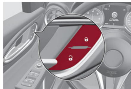
Interior Lock Switch Panel
