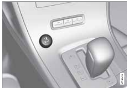
12-volt socket in the front tunnel console
