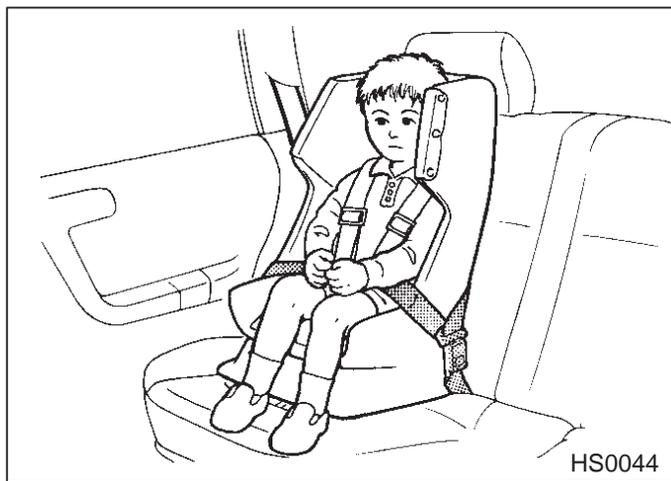
1. Adjust the seatbacks to fit the child restraint system, but as upright as possible. Make sure that the seatback is securely locked into place.
