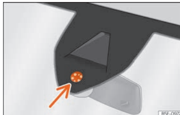
Fig. 100 Rain sensor sensitive surface
