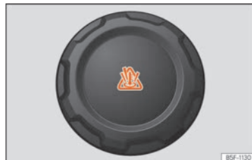
Fig. 246 Engine compartment: coolant expansion tank cap.
