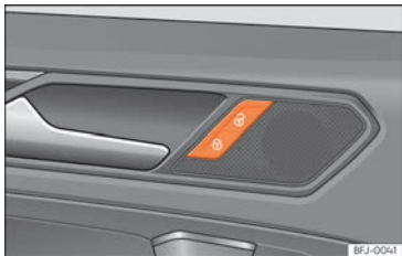
Fig. 77 Driver's door: central locking switch.
