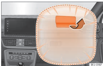
Fig. 16 Front passenger airbag located in dash panel.
