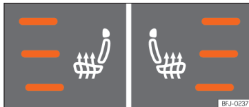
Fig. 14.8 In the centre console: front seat heating switches.
