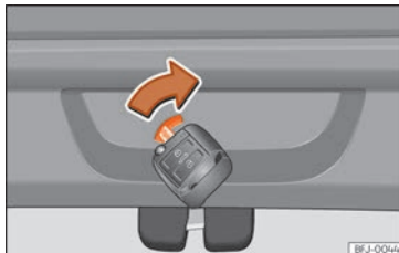
Fig. 88 Detail of the luggage compartment: emergency unlocking
