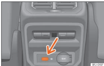
Fig. 161 Rear part of the centre console: USB connectors with power outlet function.
