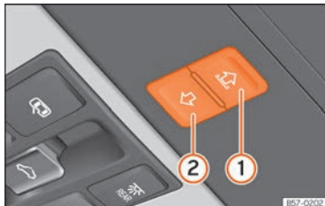
Fig. 91 On the interior roof lining: sunshade blind buttons.
