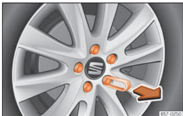
Fig. 33 Wheel: wheel nuts with caps.
