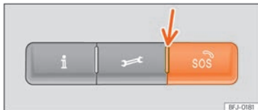
Fig. 30 On the roof console: voice service controls
