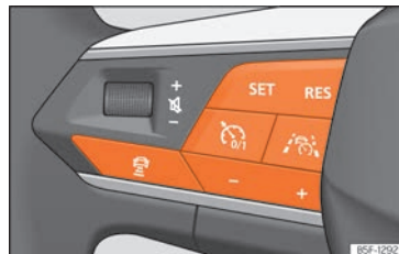
Fig. 192 Left side of the multifunction steering wheel: buttons for operating Travel Assist.
