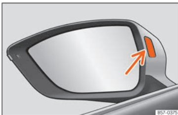
Fig. 193 Control lamp of the lane departure warning.
