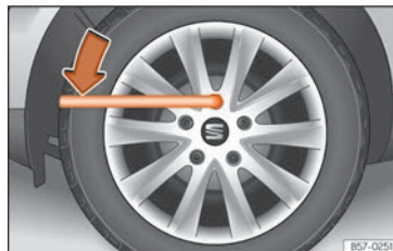
Fig. 35 Wheel change: loosen the wheel nuts.
