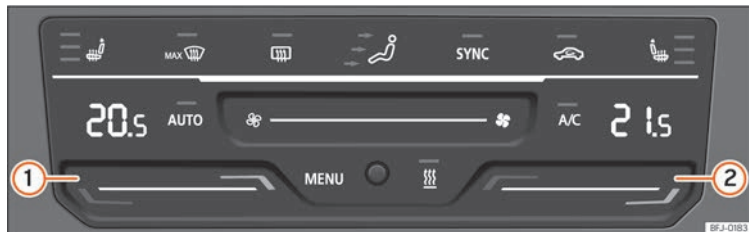
Fig. 145 In the centre console: Climatronic controls.
