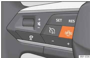
Fig. 65 Left side of the multifunction steering wheel: button for driver assistance systems (depending on versions).
