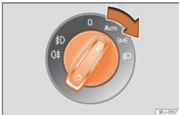
Fig. 93 Dash panel: lights control.
