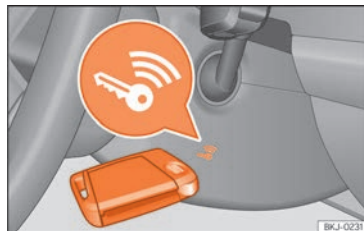
Fig. 163 On the right of the steering column: emergency start.
