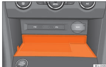
Fig. 159 In the centre console: pad for the mobile phone connection.
