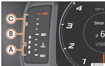
Fig. 62 Digital instrument panel: engine coolant temperature indicator.
