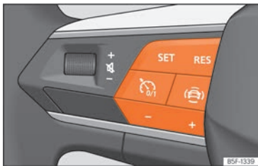
Fig. 179 On the multifunction steering wheel: buttons to operate the speed limiter.
