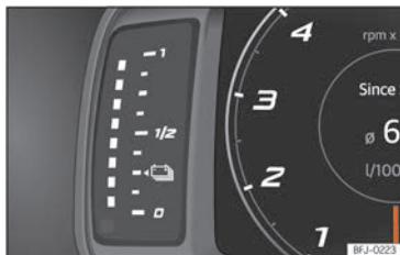
Fig. 60 Instrument panel: battery level indicator.
