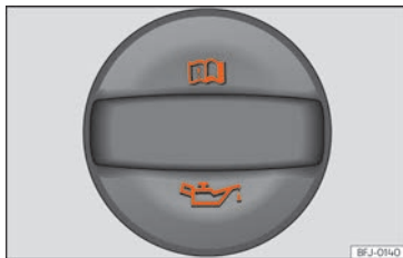
Fig. 243 In the engine compartment: Engine oil filler cap.
