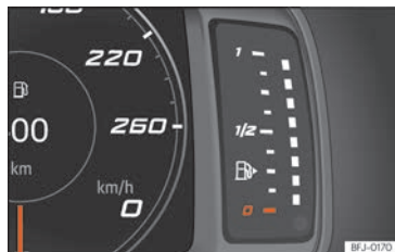
Fig. 61 Digital instrument panel: fuel gauge.
