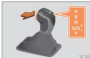
Fig. 167 Selector lever lock.
