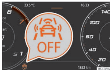
Fig. 182 On the instrument panel display: Front Assist deactivated indication.
