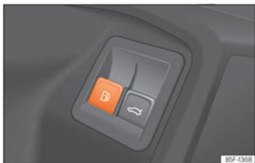
Fig. 233 Driver's door: tank flap release.
