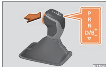
Fig. 168 Selector lever lock (hybrid vehicles).
