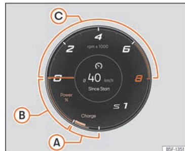
Fig. 59 Digital instrument panel: Power meter
