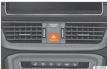
Fig. 96 Dash panel: hazard warning lights switch
