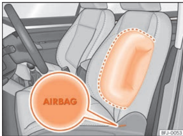
Fig. 21 Side airbag in driver's seat.
