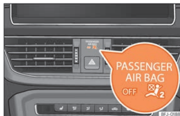
Fig. 18 Dash panel: control lamp for the deactivation of the front passenger front airbag.
