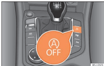
Fig. 165 Centre console: Start-stop system button.
