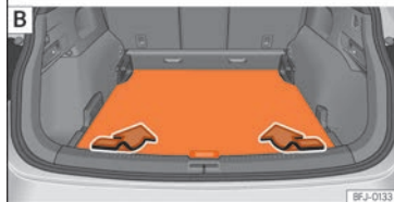
Fig. 125 In the luggage compartment: adjust the height of the variable luggage compartment floor.
