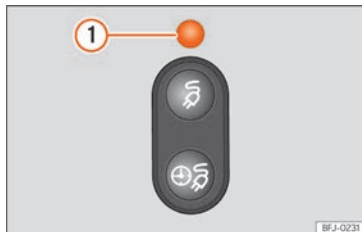
Fig. 227 Behind the cover of the battery charging socket: charging process display
