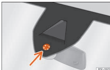
Fig. 150 Windscreen humidity and temperature sensor.
