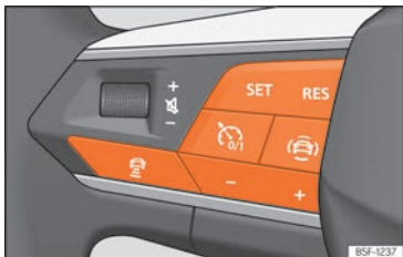
Fig. 184 On the multifunction steering wheel: buttons to operate the ACC
