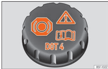
Fig. 247 Engine compartment: brake fluid reservoir cap.
