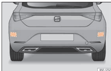
Fig. 174 Rear view of the vehicle: radar sensor zones.
