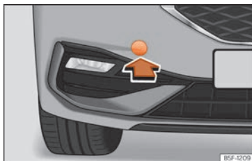
Fig. 52 On the right side of the front bumper: remove the cover.
