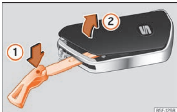
Fig. 85 Vehicle key: opening the battery compartment cover.
