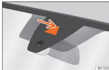
Fig. 173 On the windscreen: field of vision of the Lane Assist system.
