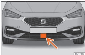
Fig. 171 On the front bumper: radar sensors.
