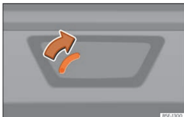
Fig. 99 Detail of the luggage compartment: manual release mechanism (Leon Sportstourer).
