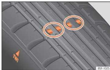
Fig. 243 Tyre profile: tread wear indicators.
