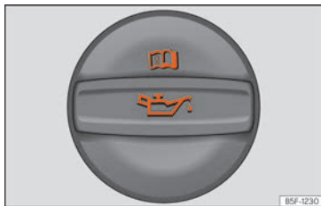
Fig. 233 In the engine compartment: Engine oil filler cap.
