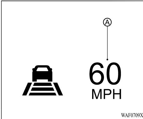
When passing another vehicle, the vehicle speed indicator Ⓐ flashes when the vehicle speed exceeds the set speed. The vehicle ahead detection indicator turns off when the area ahead of the vehicle is open. When the pedal is released, the vehicle returns to the previously set speed. Even though your vehicle speed is set in the ACC system, you can depress the accelerator pedal when it is necessary to accelerate your vehicle rapidly.
