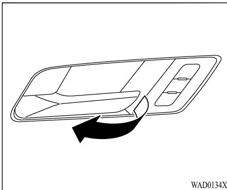
To unlock and open the driver's door, pull the door handle. To unlock and open other doors, pull once on the door handle to unlock it, and again to open it.
