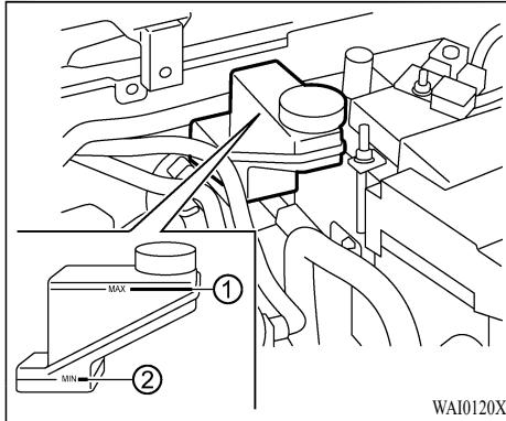
Check the fluid level in the reservoir. If the fluid is below the MIN line ② or the brake warning light comes on, add MITSUBISHI MOTORS GENUINE BRAKE FLUID SUPER4 (DOT 4) or conforming to brake fluid **DOT 3** or **DOT 4** up to the MAX line ①. If fluid must be added frequently, the system should be checked. It is recommended you visit an authorized Mitsubishi Motors dealer for this service.
