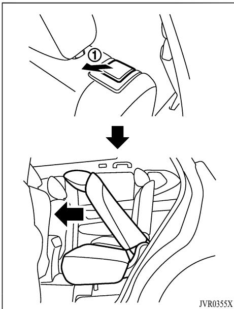
1. Pull the lever ① to tilt down the seatback.
