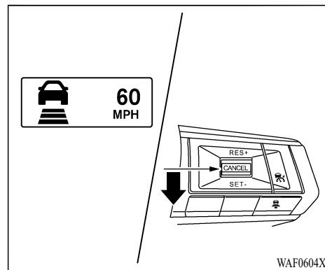
**To set cruising speed,** accelerate your vehicle to the desired speed, push the SET- switch and release it. (The vehicle ahead detection indicator, set distance indicator and set vehicle speed indicator come on.) Take your foot off the accelerator pedal. Your vehicle will maintain the set speed.
