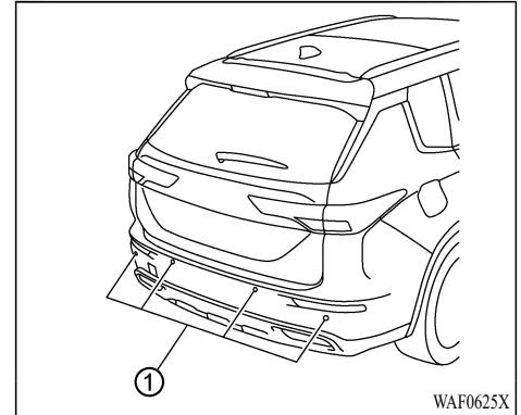
The Rear AEB system detects obstacles behind the vehicle using the rear parking sensor ① located on the rear bumper.
