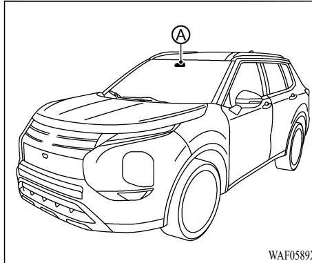
the traveling lane using the camera unit
