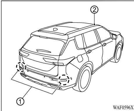
The ABSA system uses radar sensors ① installed near the rear bumper to detect other vehicles in an adjacent lane. In addition to the radar sensors, the ABSA system uses a camera ② installed behind the windshield to monitor the lane markers of your traveling lane.
