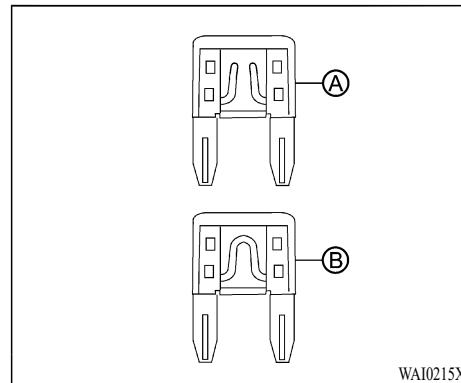
6. If the fuse is open Ⓐ, replace it with a new fuse Ⓑ.
