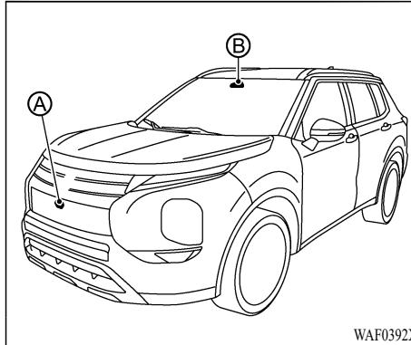
The FCM system uses a radar sensor (A) located on the front of the vehicle to measure the distance to the vehicle ahead in the same lane. For pedestrians, the FCM system uses a camera (B) installed behind the windshield in addition to the radar sensor.
