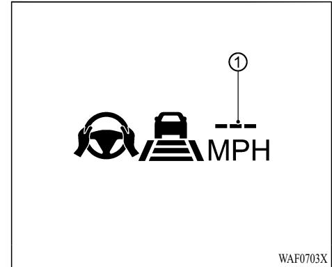
When the SET- switch is pushed down under the following conditions, the MI-PILOT Assist system cannot be set and the vehicle set speed indicator ① blinks for approximately 2 seconds and “Currently Not Available” message will appear in the multi-information display.
