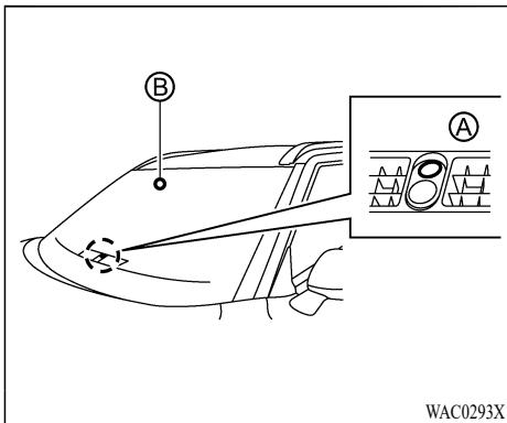
**Be sure not to put anything on top of the light sensor ① (if so equipped) located on the top of the instrument panel or rain/light sensor ② (if so equipped) located above the inside mirror. The sensor controls the Auto Headlight; if it is covered, the sensor reacts as if it is dark and the headlights will illuminate.**
