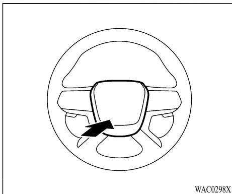
To sound the horn, push the center pad area (H) of the steering wheel.
