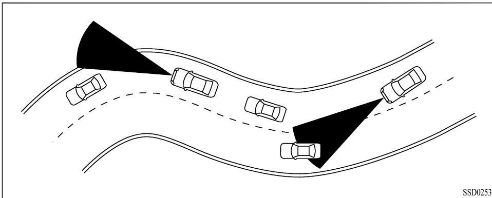
When driving on some roads, such as winding, hilly, curved, narrow roads, or roads which are under construction or on a slope, the sensor may detect vehicles in a different lane, or may temporarily not detect a vehicle traveling ahead. This may cause the system to work inappropriately.
