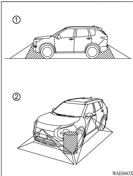
There are some areas where the system will not show objects and the system does not warn of moving objects. When in the front or the rear view display, an object below the bumper or on the ground may not be viewed ①. When in the bird's-eye view, a tall object near the seam ② of the camera viewing areas will not appear in the monitor.
