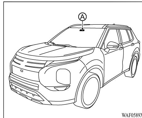
The LDW system will operate when the vehicle is driven at speeds of approximately 37 MPH (60 km/h) and above, and the lane markings are clearly visible on the road.
