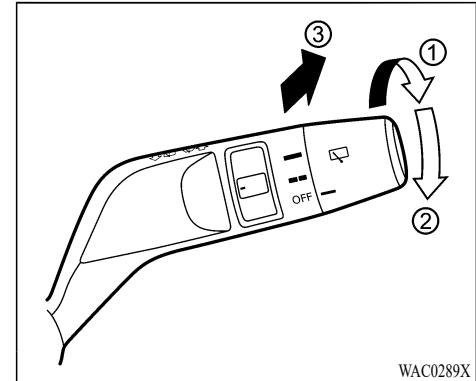
The rear window wiper and washer operate when the ignition switch is in the ON position. Turn the switch clockwise from the OFF position to operate the wiper.
