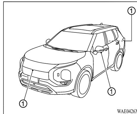
To display the multiple views, the Multi Around Monitor system uses cameras ① located in the front grille, on the vehicle's door mirrors and one just above the vehicle's license plate.
