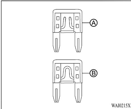
4. If the fuse is open (A), replace it with a new fuse (B).
