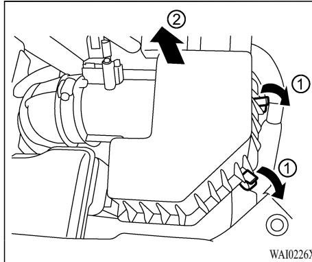
To remove the filter, release the lock pins ① and pull the unit upward ②.
