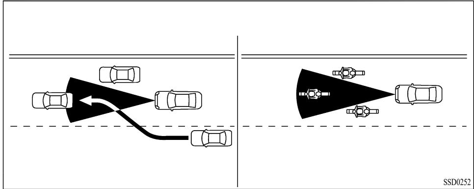
The detection zone of the ACC sensor is limited. A vehicle ahead must be in the detection zone for the vehicle-to-vehicle distance detection mode to maintain the selected distance from the vehicle ahead.
