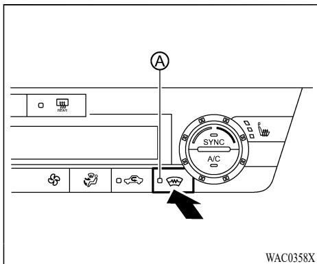
The wiper deicer switch (defroster switch) operates when the engine is running.
