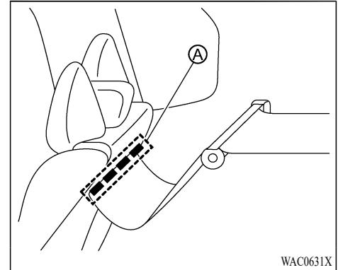
To fully cover the luggage area, affix the fasteners ① on the front cover to the back of the second row seats.
