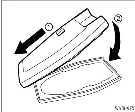
4. Align the tips of the upper and lower parts ①, and then push them together ② until it is securely closed.
