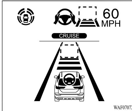
System set display — no vehicle detected ahead\*
