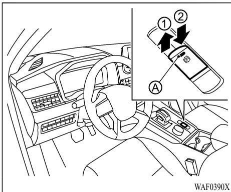
The electric parking brake can be released automatically or by operating the parking brake switch.
