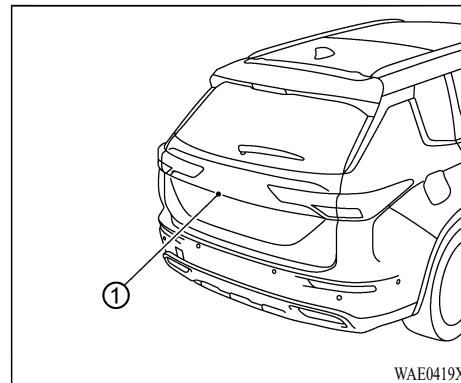
To display the rear view, the Rearview camera system uses a camera located just above the vehicle's license plate ①.
