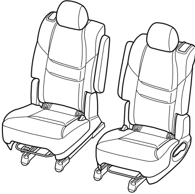
Armrest type with angle adjustment function (center walk-through)
