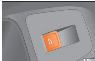
Fig. 86 On the driver's door: button to open and close the rear lid.
