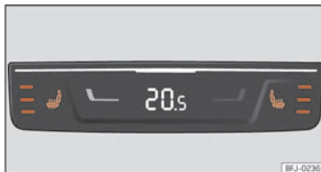
Fig. 151 In the rear part of the centre console: rear seats heating switch.
