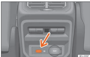
Fig. 163 Rear part of the centre console: USB connectors with power outlet function.
