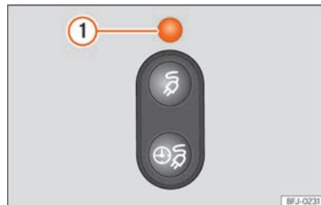
Fig. 229 Behind the cover of the battery charging socket: charging process display
