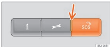
Fig. 30 On the roof console: voice service controls
