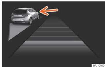
Fig. 188 On the instrument panel display: ACC active, vehicle detected in an outer lane.
