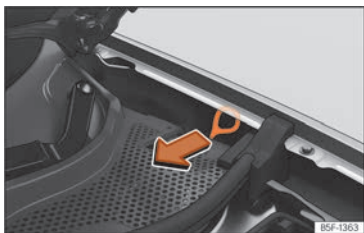
Fig. 231 Between the left wing panel and the engine bonnet hinge: Charging connector manual release mechanism puller.
