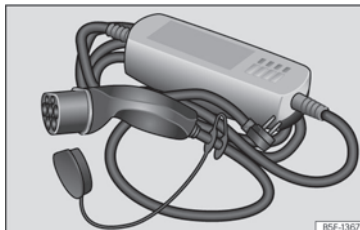
Fig. 233 Charging cable for electrical sockets
