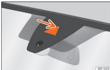
Fig. 177 On the windscreen: field of vision of the Lane Assist system.
