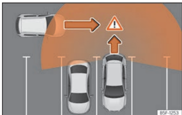
Fig. 199 Schematic representation of the rear cross traffic alert assistant: zone monitored around the vehicle while leaving a parking space.
