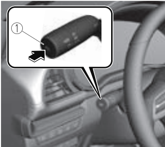
1. High beam control switch
