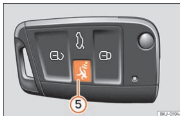
Fig. 72 Vehicle key with alarm button.
