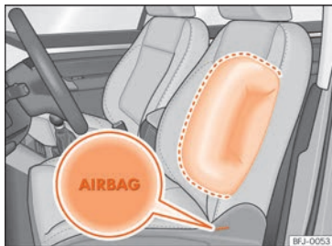
Fig. 22 Side airbag in driver's seat.
