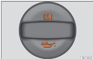
Fig. 314 In the engine compartment: Engine oil filler cap.
