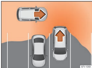
Fig. 277 Schematic representation of the rear cross traffic alert assistant: zone monitored around the vehicle while leaving a parking space.
