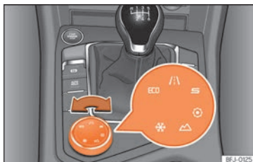
Fig. 249 Centre console: Driving Experience button.
