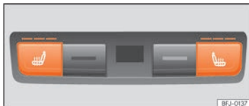
Fig. 158 In the rear part of the centre console: rear seats heating switch.
