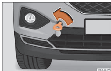
Fig. 49 On the right side of the front bumper: towline anchorage in position.
