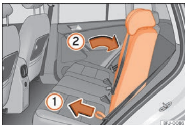
Fig. 110 Rear seat backrest adjustment.
