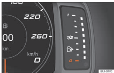
Fig. 62 Digital instrument panel: fuel gauge.
