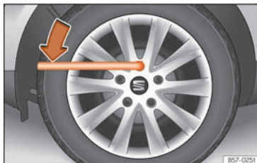
Fig. 38 Wheel change: loosen the wheel nuts.
