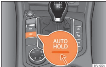
Fig. 280 In the lower part of the centre console: Auto Hold function button.
