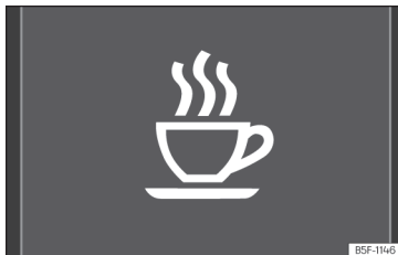
Fig. 60 On the instrument panel display: driver alert system symbol.
