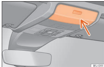
Fig. 143 On the roof console: glasses case.
