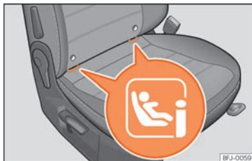
Fig. 29 Front passenger seat: ISOFIX securing rings.
