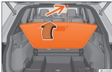
Fig. 128 In the luggage compartment: lift the luggage compartment floor.
