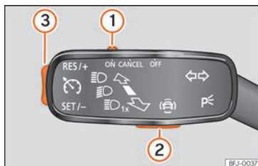
Fig. 254 On the turn signal lever: buttons to operate the speed limiter.
