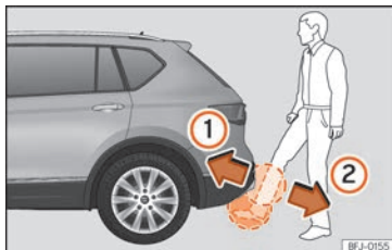
Fig. 87 Rear lid with sensor-controlled opening [Easy Open].
