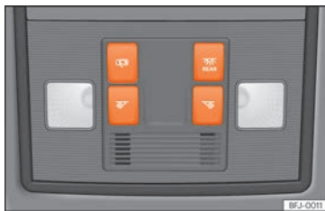
Fig. 100 Detail of roof lining: front lighting of the passenger compartment.
