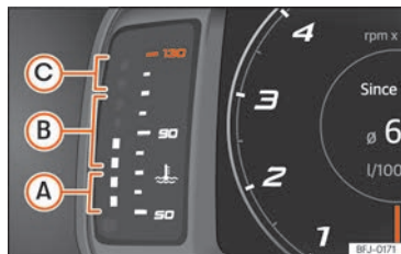
Fig. 63 Digital instrument panel: engine coolant temperature indicator.
