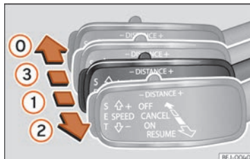
Fig. 265 On the left of the steering column: operating the ACC with the third lever.
