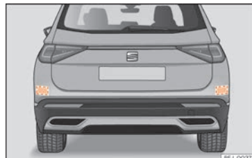
Fig. 274 Rear view of the vehicle: radar sensor zones.
