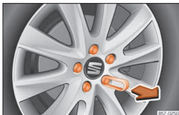
Fig. 36 Wheel: wheel nuts with caps.
