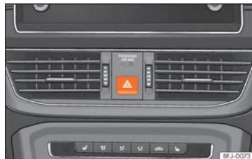
Fig. 98 Dash panel: hazard warning lights switch
