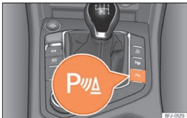
Fig. 288 Centre console: parking aid button.
