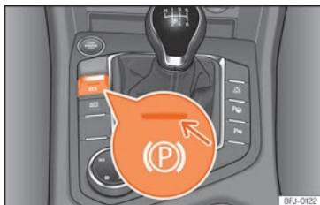
Fig. 278 In the lower part of the centre console: electronic parking brake button
