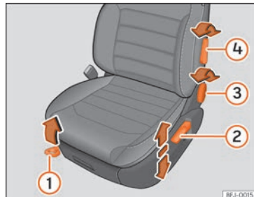
Fig. 107 Front seats: manual seat settings. »
