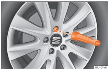
Fig. 42 Wheel change: loosen wheel nuts with the socket in the handle of the screwdriver.
