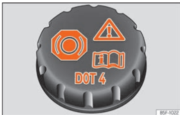
Fig. 317 Engine compartment: brake fluid reservoir cap.
