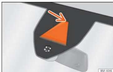
Fig. 270 On the windscreen: field of vision of the Lane Assist system.
