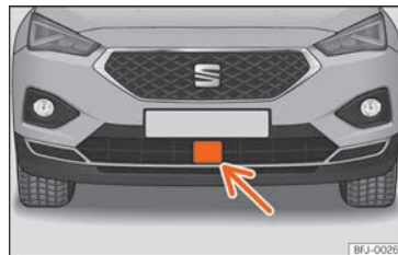
Fig. 264 On the front bumper: radar sensors.
