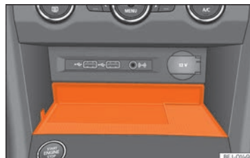
Fig. 239 In the centre console: pad for the mobile phone connection.
