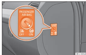
Fig. 18 Switch for activating and deactivating the front passenger airbag.
