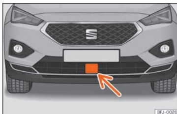
Fig. 258 On the front bumper: radar sensors.
