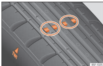
Fig. 320 Tyre profile: tread wear indicators.
