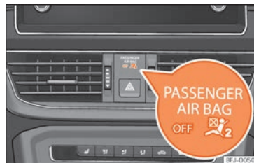
Fig. 19 Dash panel: control lamp for the deactivation of the front passenger front airbag.
