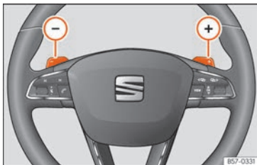
Fig. 247 Steering wheel: automatic transmission levers
