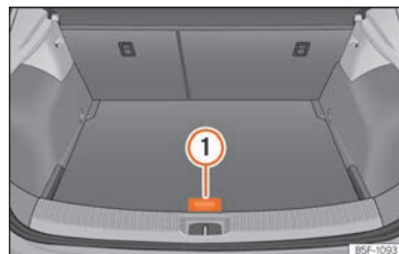
Fig. 145 Luggage compartment: adjustable floor
