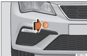
Fig. 47 On the right side of the front bumper: remove the cover.
