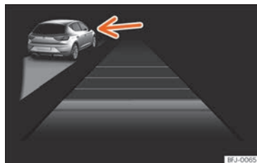
Fig. 268 On the instrument panel display: ACC active, vehicle detected in an outer lane.
