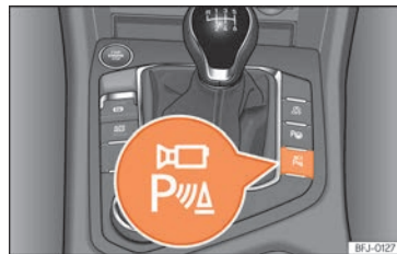
Fig. 293 Centre console: button for activating/deactivating the Area View system manually in combination with the parking aid system [(A)] or else with the rear ParkPilot system [(B)].
