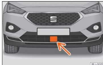
Fig. 265 On the front bumper: radar sensor.
