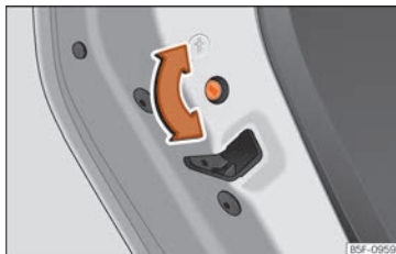
Fig. 124 Childproof lock on the left hand side door.
