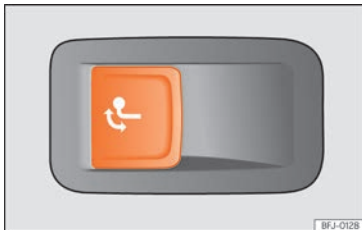
Fig. 298 Left side of the boot: button to unlock the tow hitch.
