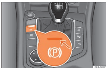
Fig. 246 Centre console, lower part: electronic parking brake button.
