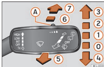
Fig. 47 Operating the windscreen wiper and rear wiper.
