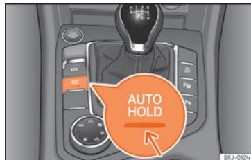
Fig. 253 In the lower part of the centre console: Auto Hold function button.
