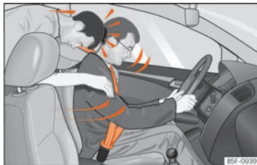
Fig. 91 The unbelted passenger in the rear seat is thrown forward violently, hitting the driver who is wearing a seat belt.
