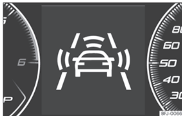
Fig. 259 On the instrument panel display: advance warning indications.
