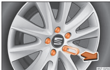
Fig. 73 Wheel: wheel bolts with caps.
