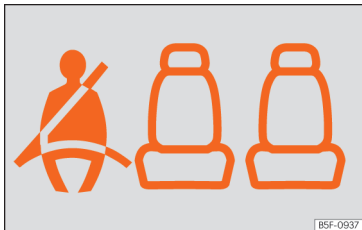
Fig. 88 Dashboard: left rear seat occupied and corresponding seat belt fastened display.
