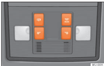
Fig. 46 Detail of headliner: front interior lighting.
