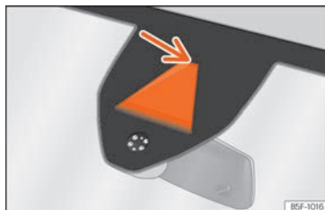
Fig. 271 On the windscreen: field of vision of the Lane Assist system camera.
