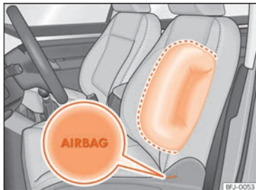
Fig. 32 Side airbag in driver's seat.
