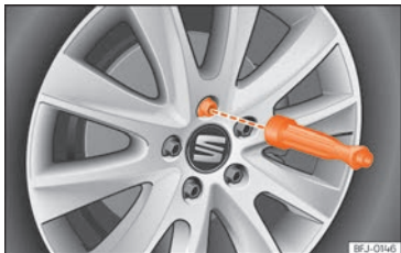
Fig. 78 Wheel: loosen wheel bolts with the socket at the end of the wheel brace
