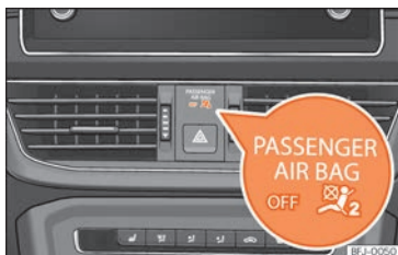
Fig. 29 Dashboard: control lamp for deactivated front passenger airbag in centre console.
