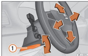
Fig. 24 Lever in the lower left side of the steering column.
