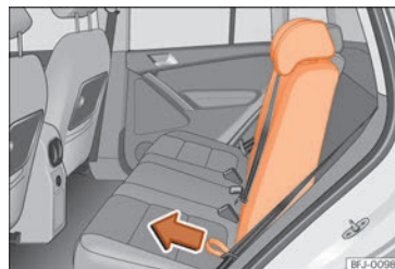
Fig. 155 Folding down and lifting the rear seat backrest
