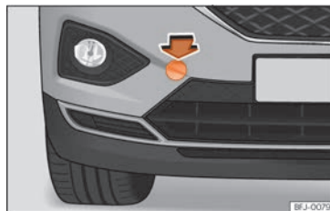
Fig. 98 Front bumper on right: remove the lid.
