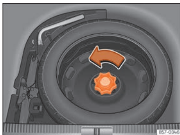
Fig. 311 Spare wheel: floor panel raised.
