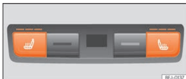
Fig. 189 In the centre console, rear section: controls for rear seat heating.
