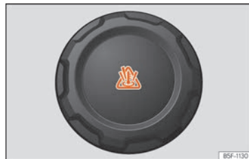
Fig. 62 Engine compartment: coolant expansion tank cap.
