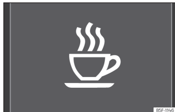
Fig. 110 On the screen of the instrument panel: fatigue detection.
