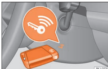
Fig. 244 On the right of the steering column: emergency start.
