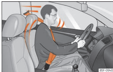
Fig. 89 Drivers with properly worn seat belts will not be thrown forward in the event of sudden braking.
