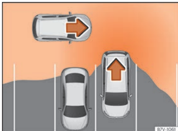
Fig. 278 Diagram of the parking assistant: detected area around the vehicle that is driving off.
