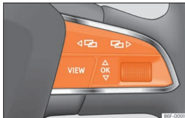
Fig. 114 Right side of multifunction steering wheel: buttons to the menus and informative indications on the instrument panel.
