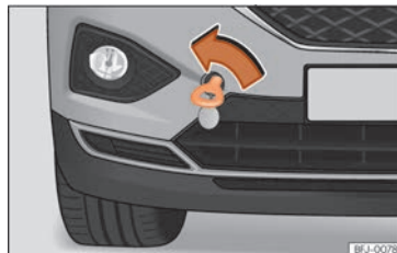
Fig. 99 Right side of the front bumper: towline anchorage screwed in.
