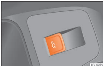
Fig. 126 Driver door: button to open and close rear lid.
