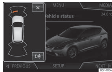
Fig. 286 Miniature indication of automatic activation.
