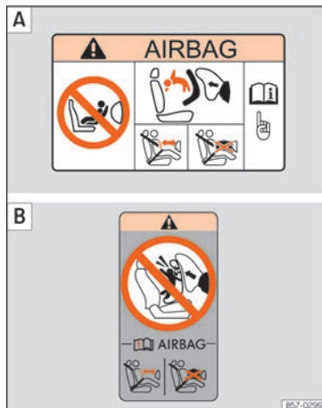
Fig. 36 Airbag adhesives - version 1: on the passenger-side sun blind A and on the rear frame of the front passenger's door B .
