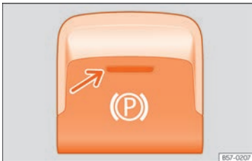
Fig. 255 Centre console, lower part: electronic parking brake button.
