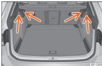
Fig. 188 In the boot: retaining hooks (LEON ST).
