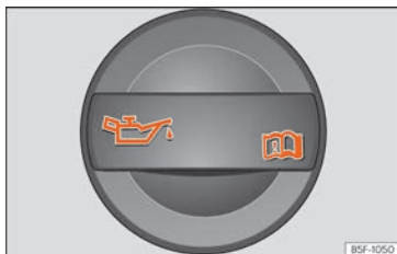
Fig. 311 In the engine compartment: Engine oil filler cap.
