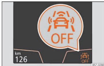
Fig. 267 On the screen of the instrument panel Front Assist switched off message.
