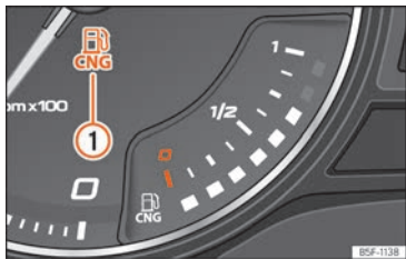
Fig. 133 Analogue instrument panel: natural gas gauge
