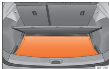
Fig. 176 In the boot: fitting the rear shelf.
