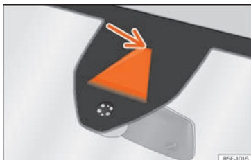
Fig. 277 On the windscreen: field of vision of the Lane Assist system camera.
