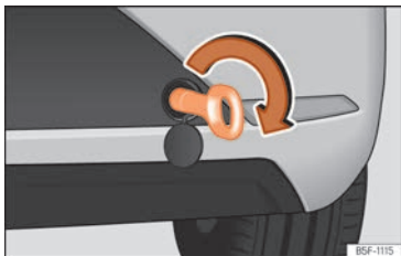
Fig. 81 Right side of the rear bumper: towline anchorage screwed in.
