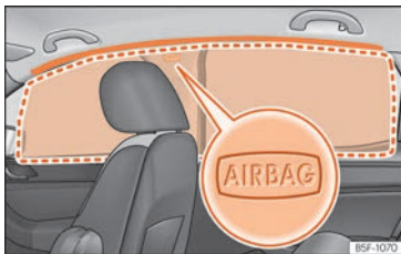
Fig. 34 Location of head-protection airbags.
