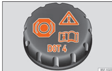
Fig. 65 Engine compartment: brake fluid reservoir cap.
