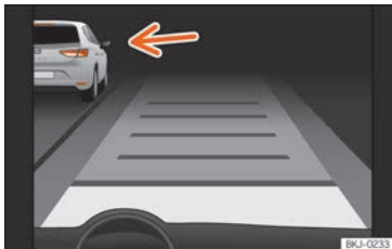
Fig. 274 On the instrument panel display: ACC active, vehicle detected in an outer lane.
