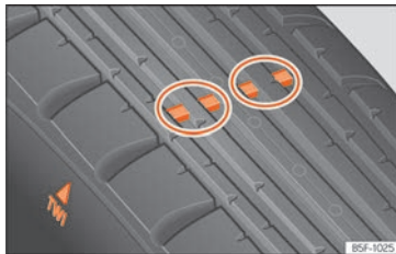
Fig. 313 Tyre profile: tread wear indicators.
