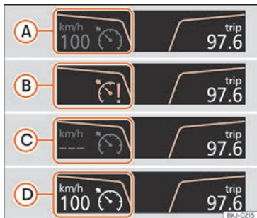
Fig. 264 Instrument panel display: CCS status indications.
