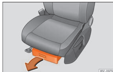
Fig. 165 Storage compartment under the front seats.
