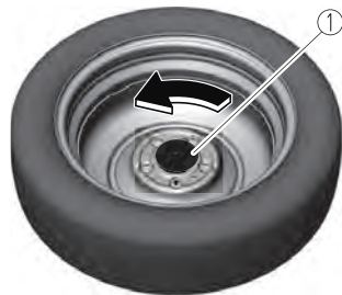
1. Spare tire hold-down bolt
