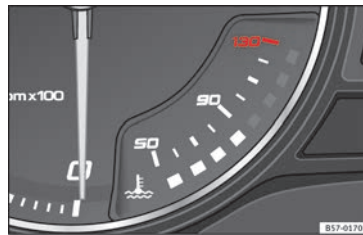
Fig. 124 Instrument panel: coolant temperature gauge
