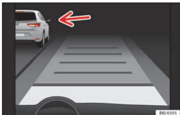
Fig. 213 On the instrument panel display: ACC active, vehicle detected in an outer lane.
