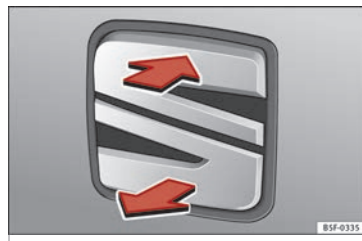
Fig. 5 Rear lid: opening from the outside.
