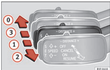
Fig. 211 On the left of the steering column: third lever for operating the Adaptive Cruise Control.
