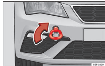
Fig. 77 Right side of the front bumper: towline anchorage screwed in.
