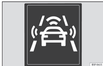
Fig. 204 On the instrument panel display: pre-warning messages.
