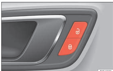
Fig. 2 Driver door: central locking switch.
