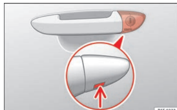
Fig. 3 Driver door lever: hidden lock cylinder.
