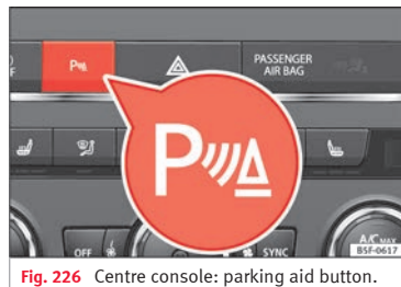
Fig. 226 Centre console: parking aid button.
