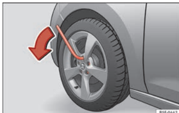
Fig. 74 Wheel: loosen the wheel bolts.
