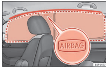
Fig. 28 Location of head-protection airbags.
