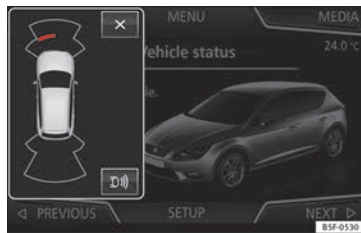
Fig. 227 Miniature indication of automatic activation.
