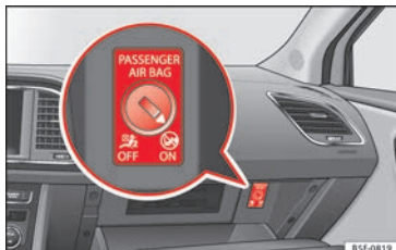
Fig. 22 Front passenger front airbag switch.
