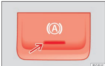
Fig. 202 In the lower part of the centre console: Auto Hold function button.
