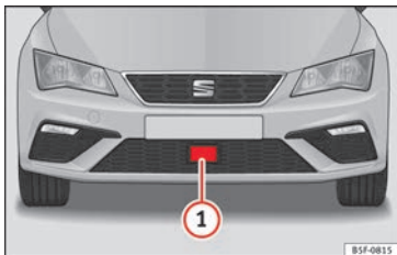
Fig. 210 On the front bumper: radar sensor.
