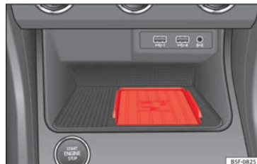
Fig. 131 Centre console: Connectivity Box.
