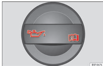
Fig. 249 In the engine compartment: Engine oil filler cap.
