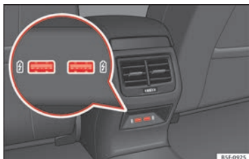
Fig. 129 Centre console, rear section: USB connectors.
