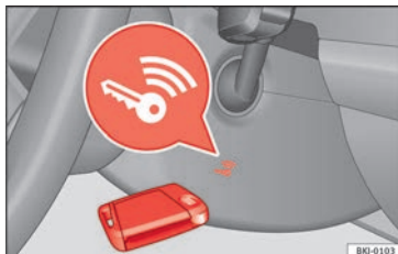
Fig. 193 On the right of the steering column: emergency start.
