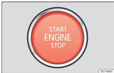
Fig. 192 In the lower part of the centre console: starter button.
