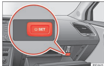
Fig. 254 Glove compartment: tyre control switch.
