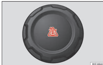
Fig. 63 Engine compartment: coolant expansion tank cap.
