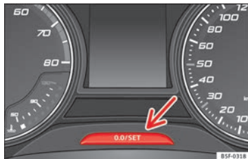
Fig. 123 Instrument panel: odometer and reset button.
