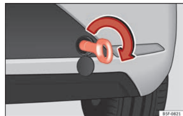
Fig. 78 Right side of the rear bumper: towline anchorage screwed in. »
