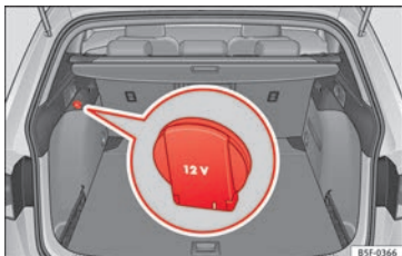
Fig. 162 Detailed view of the side trim in the luggage compartment: 12-volt power socket (applies only to the LEON ST model).
