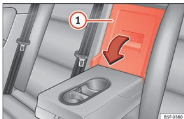
Fig. 175 On the rear seat backrest: opening the tailboard.
