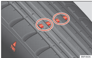
Fig. 251 Tyre tread: tread wear indicators
