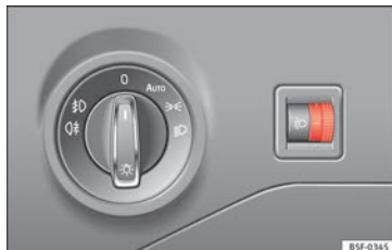
Fig. 144 Next to the steering wheel: Headlight range control
