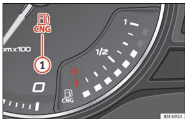
Fig. 126 Instrument panel: Natural gas gauge
