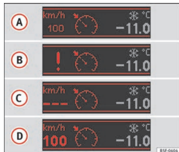
Fig. 203 Instrument panel display: CCS status indications.
