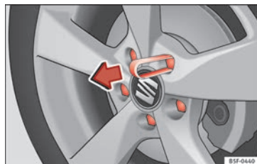
Fig. 72 Wheel: wheel bolts with caps.
