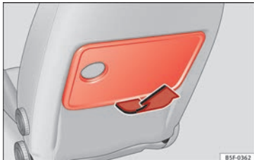
Fig. 158 Left-hand front seat: folding table.
