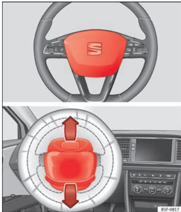
Fig. 20 Driver airbag located in steering wheel.
