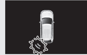
Example: Corner sensor (left) malfunctioning
