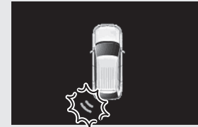
Example: Corner sensor (left) malfunctioning
