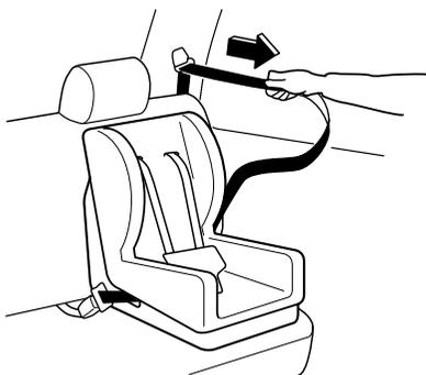
3. Push the child-restraint system firmly into the vehicle seat. Be sure the belt retracts as snugly as possible. Clicking from the retractor will be heard during retraction if the system is in the automatic locking mode. If the belt does not lock the seat down tight, repeat this step.
