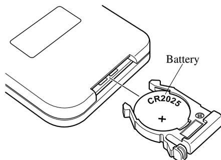
3. Press the battery case tab in the direction of the arrow until a click sound is heard.
