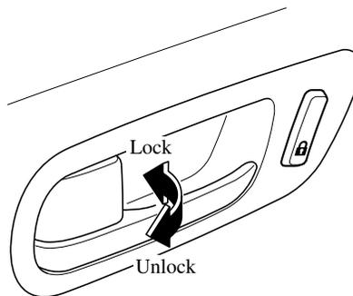
To lock any door with the door-lock knob from the outside, push the door-lock knob to the lock position and close the door.
