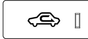
Outside or recirculated air positions can be selected. Press the switch to select outside/recirculated air positions.
