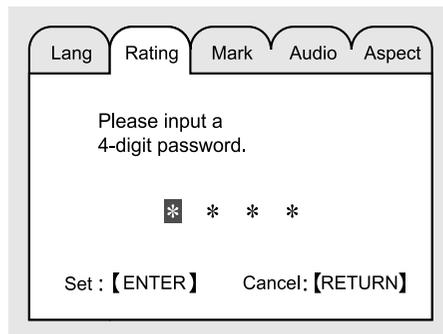
2. Press the ENTER button. If the password is confirmed, the Rating change mode is displayed.
