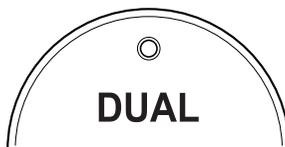
Use the DUAL switch to change the mode between the individual operation and interconnection modes.
