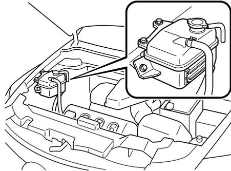
If it's at or near L, add enough coolant to the coolant reservoir to provide freezing and corrosion protection and to bring the level to F.
