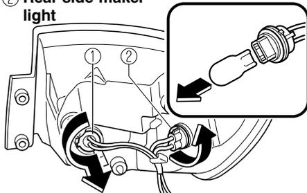
4. Disconnect the bulb from the socket.
