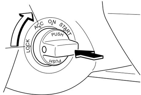
9. Turn the ignition switch from the ACC position to the START position and hold (up to 10 seconds at a time) until the engine starts.
