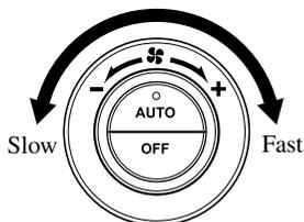
The fan has seven speeds. The selected speed will be displayed.
