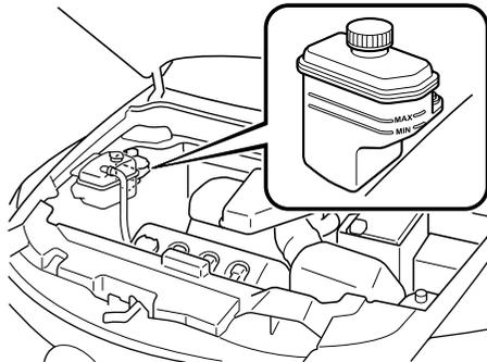
The level must be kept between MAX and MIN.
