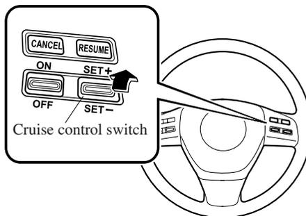
Your vehicle has a tap-up feature that allows you to increase your current speed in increments of 1.6 km/h (1 mph) by a momentary tap of the cruise control switch. Multiple taps will increase your vehicle speed 1.6 km/h (1 mph) for each tap.
