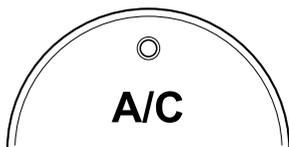
With the AUTO or fan control dial ON, press the A/C switch to turn the air conditioning (cooling/dehumidifying functions) on or off.
