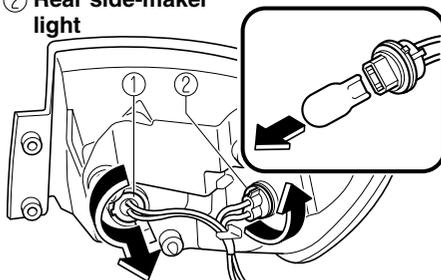
4. Disconnect the bulb from the socket.
