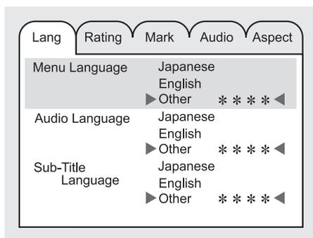
2. Move the cursor to the desired menu by operating the select button up/down or left/right.
