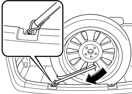
12. Pull the belt end to secure the flat tire.
