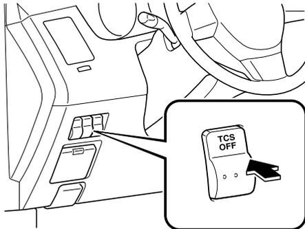
Press the switch again to turn the TCS back on. The TCS OFF indicator light will go out. If the vehicle speed is more than 15 km/h (9 mph), the TCS OFF indicator light will not illuminate even if the switch is pressed.
