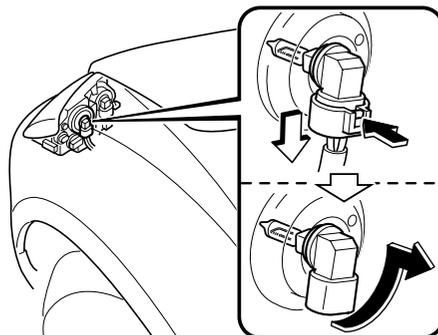
7. Install the new bulb in the reverse order of removal.
