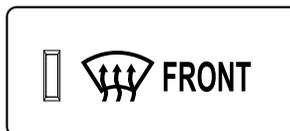
Press the windshield defroster switch. In this position, the
