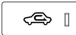
Outside or recirculated air positions can be selected. Press the switch to select outside/recirculated air positions.
