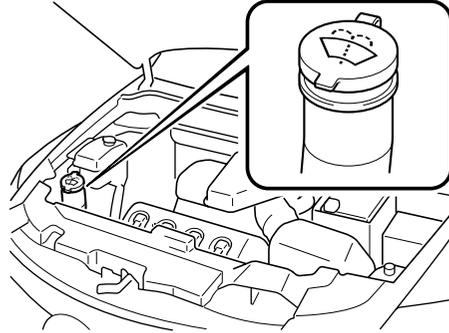
Use plain water if washer fluid is unavailable. But use only washer fluid in cold weather to prevent it from freezing.
