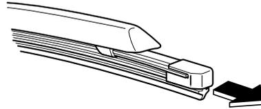
6. Remove the metal stiffeners from each blade rubber and install them in the new blade.
