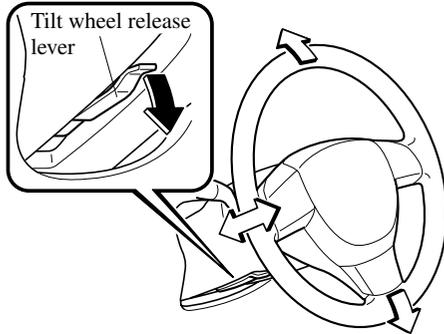
2. Tilt the steering wheel and/or adjust the steering column length to the desired positions, push the lever up to lock the column.
