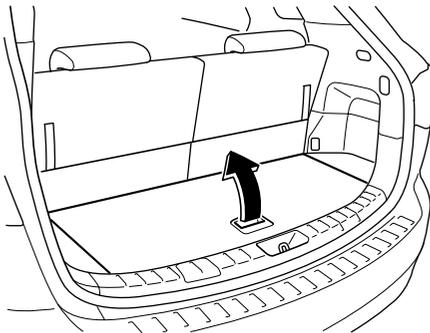
2. Secure the trunk board using the straps on the third-row seatbacks.
