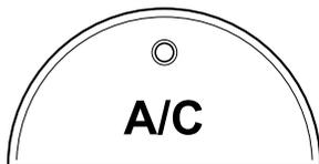
With the AUTO or fan control dial ON, press the A/C switch to turn the air conditioning (cooling/dehumidifying functions) on or off.
