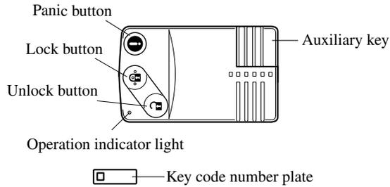
A code number is stamped on the plate attached to the key set; detach this plate and store it in a safe place (not in the vehicle) for use if you need to make a replacement key.
