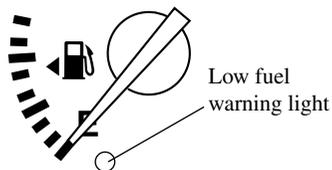
This warning light in the fuel gauge signals that the fuel tank will soon be empty.
