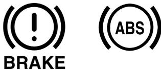
If the electronic brake force distribution control unit determines that some components are operating incorrectly, the control unit may turn the brake system warning light and the ABS warning light on at the same time. The problem is likely to be an electronic brake force distribution system.
