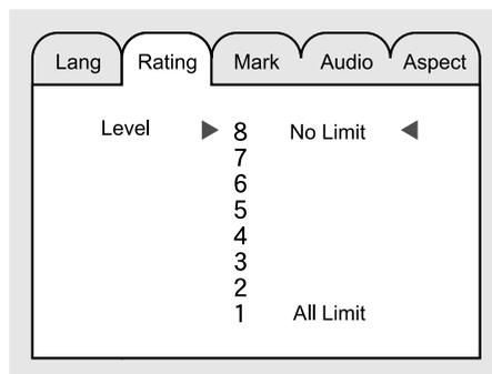
3. Select the desired parent lock level and press the ENTER button to set.
