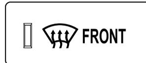
Press the switch to defrost the windshield and front door windows.
