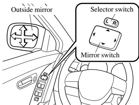
After adjusting the mirror, lock the control by placing the selector switch in the middle position.
