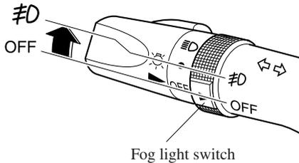
To turn them off, rotate the fog light switch to the OFF position or turn the headlight switch to the  $\bullet$  or OFF position.
