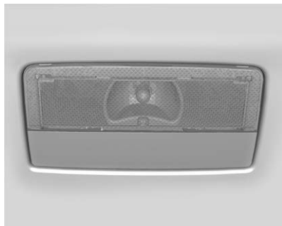
Center Dome Lamp
