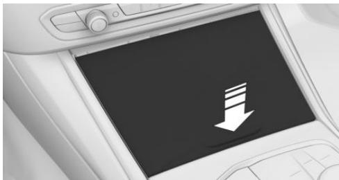
2. A socket is located between the cup holders. Detach the cover.
