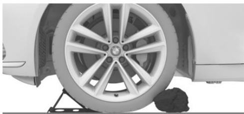
Place wheel chocks or other suitable objects in front and behind the wheel that is diagonal to the wheel to be changed.
