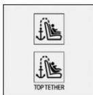
The respective icon shows the attachment point for the upper retaining strap. Seats with an upper top tether are marked with this icon. It is located on the rear seat backrest, the rear shelf or the rear seat.
