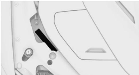
The engraved vehicle identification number can be found under the hood on the right-hand side of the vehicle.
