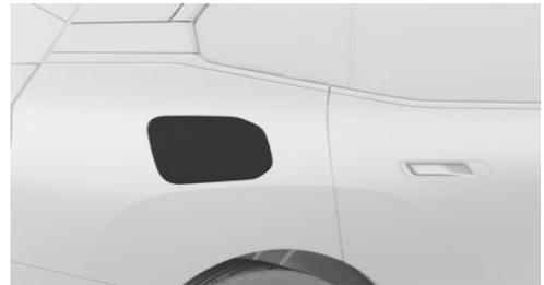
The charging socket cover is located in the rear on the right side of the vehicle.
