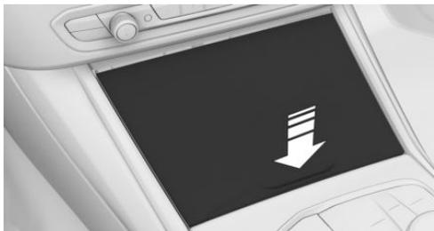
2. The ashtray is located in a cup holder. Fold the ashtray cover upward.
