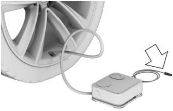
5. With standby or drive readiness turned on, turn on the compressor and let it run for a maximum of 10 minutes.
