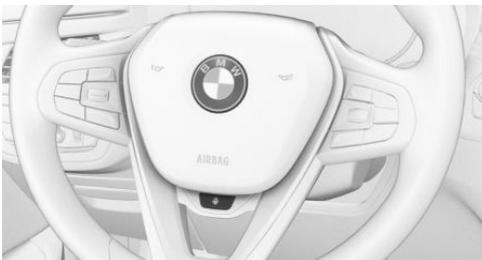
Button for steering wheel heating
