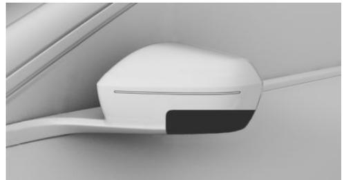
One camera is located at the bottom of each exterior mirror housing.
