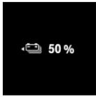
When standby and drive readiness are turned on, the available battery charge state of the high-voltage battery is continuously displayed in percent in the instrument cluster.
