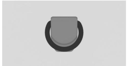
There are several lashing eyes in the cargo area for securing cargo. Attach auxiliary materials to secure the cargo such as lashing straps, tensioning straps, draw straps, or cargo nets to the lashing eyes.
