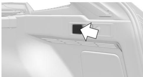
Depending on vehicle equipment, there is a socket in the cargo area on the right side. Unfold the cover.
