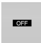
The lettering OFF in the instrument cluster indicates that drive-ready state is switched off and standby state is switched on.
