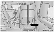
Tether Strap Anchorages (Second Row 7 Passenger Stow 'n Go Anchorage Shown)
