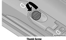
Bend the crossbar supports at each end, taking care to keep hand clear of pivoting joint. Slide the thumb screw down.
