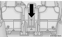
Tether Strap Anchorages (Second Row 8 Passenger Anchorage Shown)
