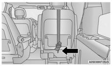
Rear Seat Tether Strap Attachment (Second Row 7 Passenger Stow 'n Go Anchorage Shown)
