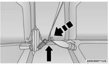
Latch Plate And Buckle Connected
