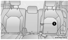
**Routing The Rear Seat Belt Latch Plate**
