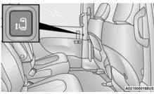
Power Sliding Side Door Switch (Left Side Shown)
