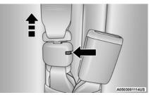
Insert Regular Latch Plate Into Mini-Buckle Slot To Detach
