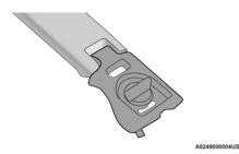
4. Once the crossbar is in place, tighten both thumb screws completely.
