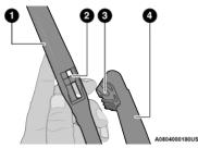
Wiper Blade Removed From Wiper Arm
