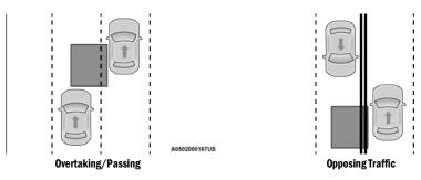
The BSM system is designed not to issue an alert on stationary objects such as guardrails, posts, walls, foliage, berms, snow banks, car washes, etc. However, occasionally the system may alert on such objects. This is normal operation and your vehicle does not require service.
