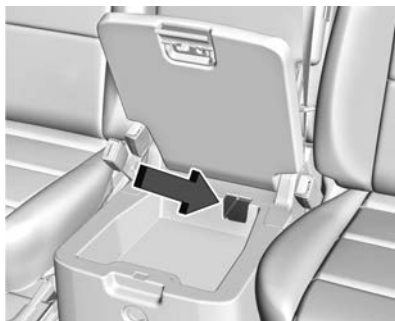
Transmitter Pocket without Bucket Seats (Lower Compartment)
