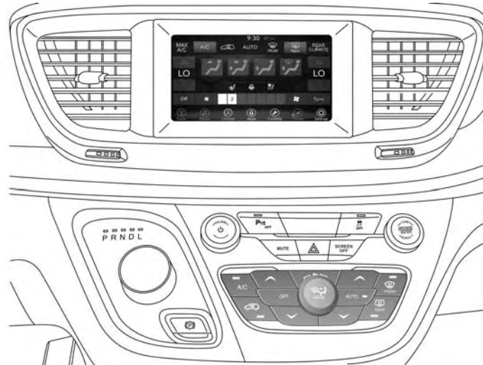
Uconnect 4 With 7-inch Display Automatic Temperature Controls
