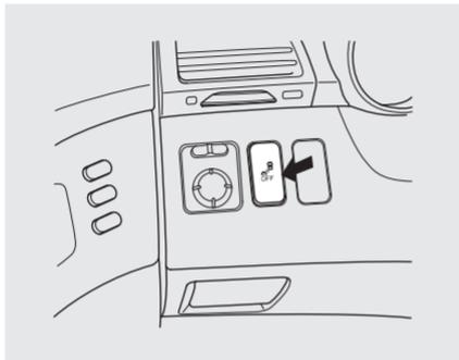
To turn the system off, press the BSI OFF button when the ignition switch is in the ON (II) position. The BSI indicator on the instrument panel glows amber, indicating that the system is turned off. The multi-information display indicates that the system is off.
