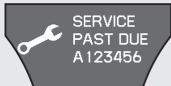
If the indicated maintenance service is not done and the remaining engine oil life reaches 0%, the multi-information display will show the message “SERVICE PAST DUE” and the maintenance item code(s). This message is displayed again when the total distance traveled is less than 10 miles (for U.S. models) or 10 km (for Canadian models) after the engine oil life became 0%.
