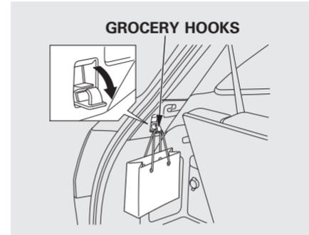
Your vehicle also has a grocery hook on each side panel in the cargo area. They are designed to hold light items. Heavy objects may damage the hook. Make sure any items put on each hook weigh less than 6.5 lbs (3 kg).
