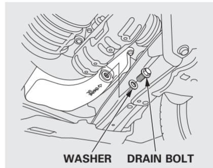
2. Open the hood, and remove the engine oil fill cap. Remove the oil drain bolt and washer from the bottom of the engine. Drain the oil into an appropriate container.
