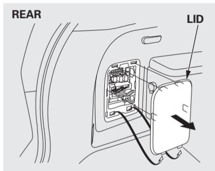
The rear fuse box is located at the left side of the cargo area.
