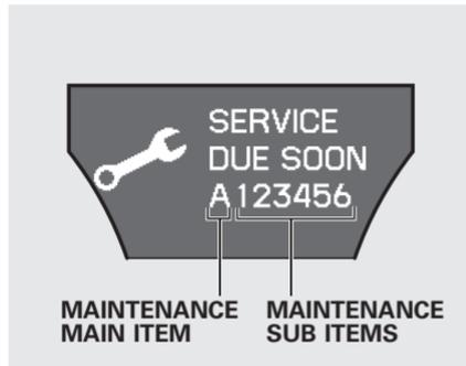
When the remaining engine oil life is 15 to 6 percent, the multi-information display shows a “SERVICE DUE SOON” message along with the maintenance schedule code indicating the main and sub items required at the time of the oil change. Refer to page 508 for a complete list of the maintenance main items and sub items.
