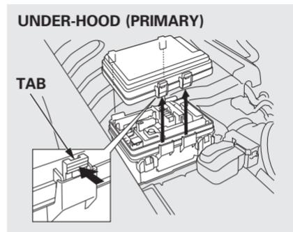
The primary under-hood fuse box is located next to the battery.
