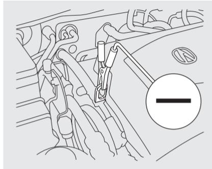
4. Connect the second jumper cable to the negative (-) terminal on the booster battery. Connect the other end to the grounding point as shown. Do not connect this jumper cable to any other part of the engine.
