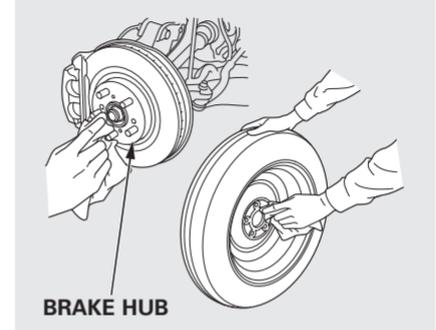
15. Before mounting the spare tire, wipe any dirt off the mounting surface of the wheel and hub with a clean cloth. Wipe the hub carefully; it may be hot from driving.
