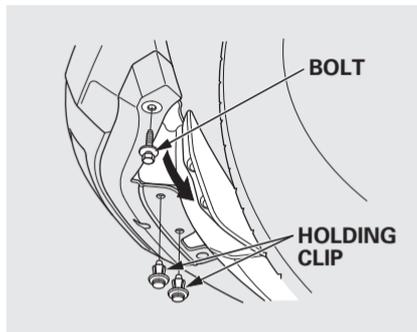
2. Remove the bolt and use the flat-tip screwdriver to remove the holding clips located under the front bumper.
