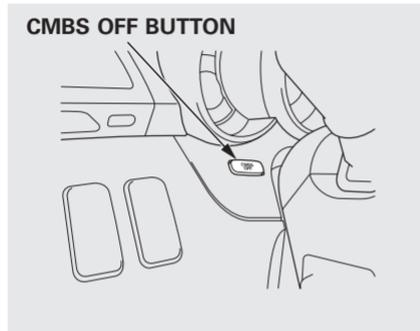
To switch the CMBS off, press the CMBS OFF button on the dashboard for about 1 second. When you do this, a beeper sounds, a CMBS indicator on the instrument panel comes on, and a CMBS OFF message appears on the multi-information display. To switch the system back on, press the button again for about 1 second.
