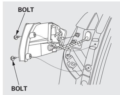
2. Remove the two bolts, and remove the rear light assembly from the rear pillar.
