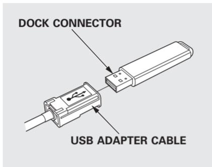
2. Connect the USB flash memory device to the USB adapter cable correctly and securely.
