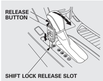
4. Insert a key into the shift lock release slot.
