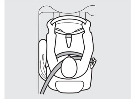
If you ever have a moderate to severe side impact, sensors will detect rapid acceleration and signal the control unit to instantly inflate either the driver's or the passenger's side airbag and activate the seat belt tensioner on the affected side.
