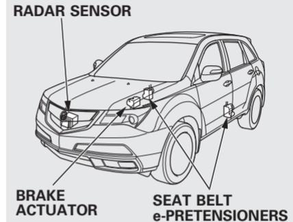
The CMBS consists of a radar sensor in the front grille, a brake actuator in the engine compartment, an indicator on the instrument panel, seat belt e-pretensioners on the front seats, and an on/off button on the dashboard.
