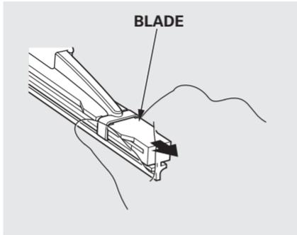
3. Remove the blade from its holder by grabbing the tabbed end of the blade. Pull firmly until the tabs come out of the holder.
