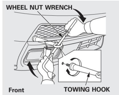
3. Screw the towing hook into the hole, and tighten it with the wheel nut wrench.
