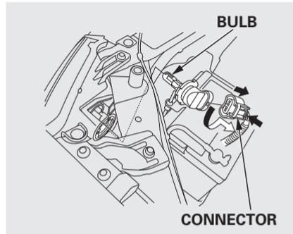
3. Remove the electrical connector from the bulb by pushing on the tab and pulling the connector down.
