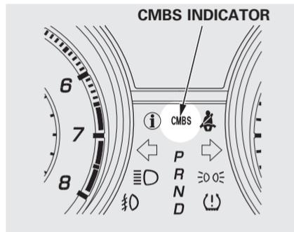
This indicator comes on for several seconds when you turn the ignition switch to the ON (II) position. It also comes on and stays on when you turn the CMBS off by pressing the CMBS OFF button.
