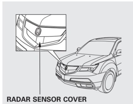
The radar sensor is located under the Acura emblem in the front grille. If the radar sensor cover is covered with mud, dirt, dead leaves, wet snow, etc., or if you put a sticker on it, the CMBS will automatically shut off, and the CMBS indicator on the instrument panel will come on. You will also see a “CHECK CMBS RADAR SENSOR” message on the multi-information display for about 5 seconds.
