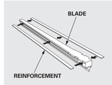
3. Examine the new wiper blades. If they have no plastic or metal edge reinforcement along the back edge, remove the metal reinforcement strips from the old wiper blade, and install them in the slots along the edge of the new blade.
