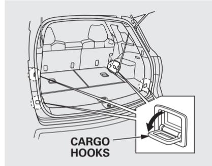
The four hooks on the side panels can be used to install a net for securing items. Each hook is designed to hold up to 50 lbs (23 kg) of weight.
