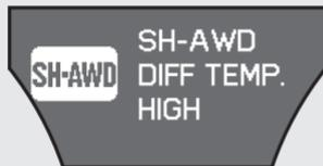
If the SH-AWD indicator blinks while driving, it indicates the differential temperature is too high. You will also see an “SH-AWD DIFF TEMP. HIGH” message on the multi-information display. If this happens, pull to the side of the road when it is safe, shift to Park, and let the engine idle until the indicator goes out. If the indicator does not go out, take your vehicle to a dealer to have it checked.
