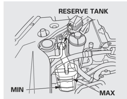
Look at the coolant level in the radiator reserve tank. Make sure it is between the MAX and MIN lines. If it is below the MIN line, see **Adding Engine Coolant** on page 514 for information on adding the proper coolant.
