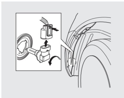
5. Remove the electrical connector from the bulb by pushing on the tab and pulling the connector down.
