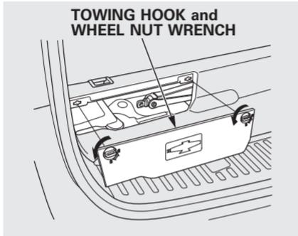
2. Remove the towing hook and wheel nut wrench located behind the cargo area cover on the driver's side.
