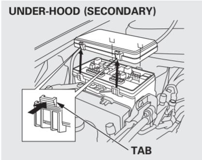
The secondary fuse box is on the passenger's side.
