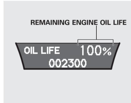
To see the remaining engine oil life displayed on the multi-information display as a percentage, turn the ignition switch to the ON (II) position. Make sure the display shows blank, SH-AWD and tire pressure, and then press the SEL/RESET button on the steering wheel repeatedly until the engine oil life appears (see page 77).
