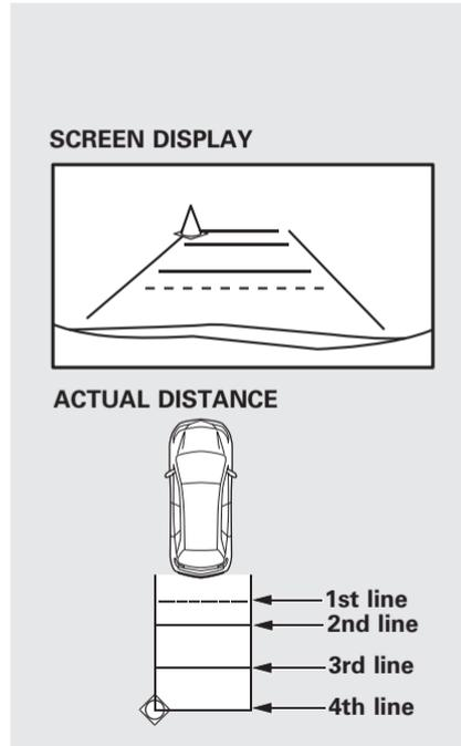
The camera display has parking guide lines that indicate distance from your vehicle.
