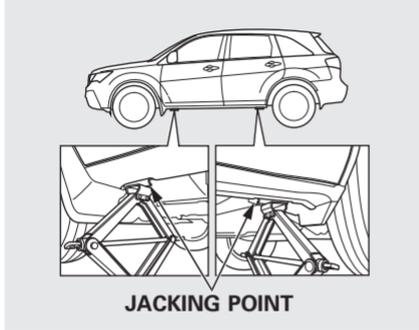
12. Place the jack under the jacking point nearest the tire you need to change. Turn the end bracket clockwise until the top of the jack contacts the jacking point. Make sure the jacking point tab is resting in the jack notch.
