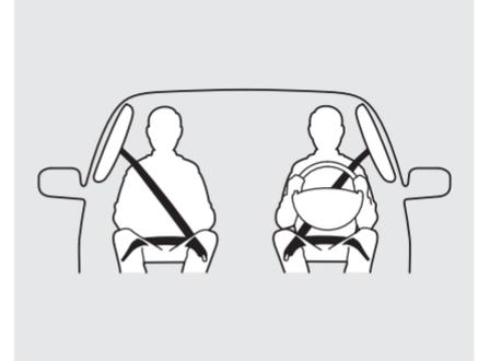
In addition, your vehicle has side curtain airbags to help protect the heads of the driver, front passenger, and passengers in the outer rear seating positions during a moderate to severe side impact or rollover (see page [34](#) for more information on how your side curtain airbags work).
