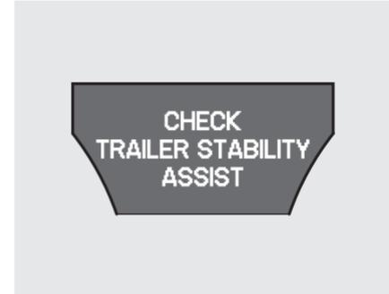
The control unit monitors the VSA circuitry and the braking system. If there is a problem with the brake lighting system, the trailer stability assist function shuts down and the “CHECK TRAILER STABILITY ASSIST” message appears on the multi-information display.
