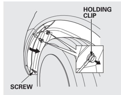
3. Use a flat-tip screwdriver to remove the holding clip from the inner fender, and remove the screw with a Phillips-head screwdriver.
