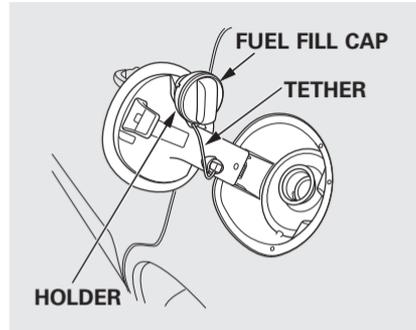
3. Remove the fuel fill cap slowly. You may hear a hissing sound as pressure inside the tank equalizes. Place the cap in the holder on the fuel fill door.
