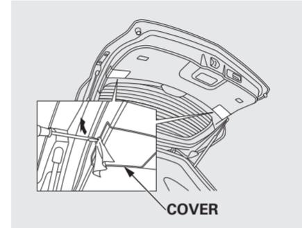
1. Open the tailgate. Place a cloth on the edge of the light assembly cover. Remove the cover by carefully prying in the notch on its middle edge with a flat-tip screwdriver.
