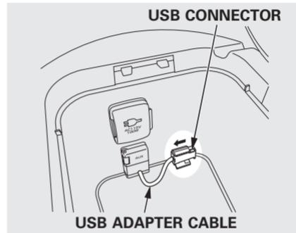
1. Unclip the USB connector by pulling it up, and pull out the USB adapter cable in the console compartment.
