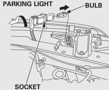
5. Push the new bulb straight into the socket until it bottoms.
