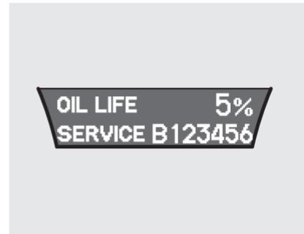
Press the SEL/RESET button on the steering wheel repeatedly to select the engine oil life. The message “SERVICE”, along with “5%”, and the maintenance item code are displayed on the lower part of the multi-information display when the calculated engine oil life is 1 – 5 percent (see page 501).
