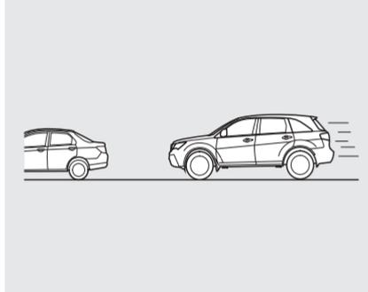
If the system senses a likely collision with a vehicle or object ahead of you, it alerts you with a visual alert or a combination of a visual alert and an audible alert.
