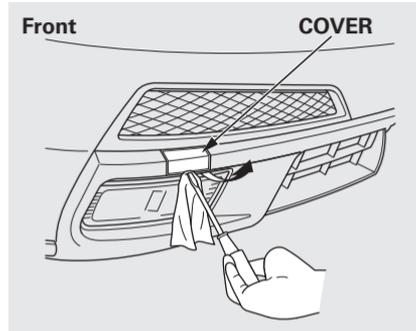
1. To remove the cover, put cloth on the edge of the cover and carefully pry with a small flat-tip screwdriver or a metal fingernail file.
