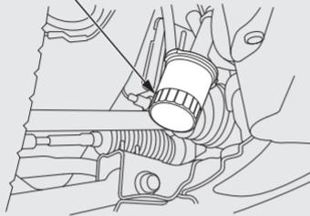
3. Remove the oil filter, and let the remaining oil drain. A special wrench (available from your dealer) is required.
