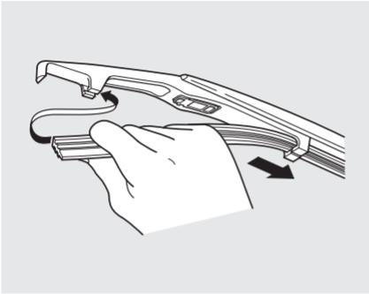
4. Slide the new blade into the wiper arm. Make sure it is engaged in the slot along its full length.
