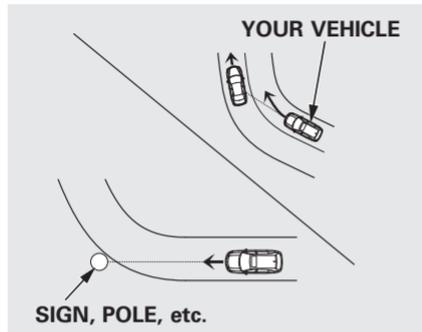
Because of the road condition (curved, winding, etc.) or the state of your vehicle (turning angle, lane position, etc.), CMBS can sometimes mistake a stationary object (light pole, traffic sign, guard rail, etc.) as a vehicle ahead of you and temporarily operate. This is normal.
