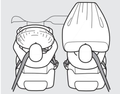
Your vehicle has a supplemental restraint system (SRS) with front airbags to help protect the heads and chests of the driver and a front seat passenger during a moderate to severe frontal collision (see page [29](#) for more information on how your front airbags work).
