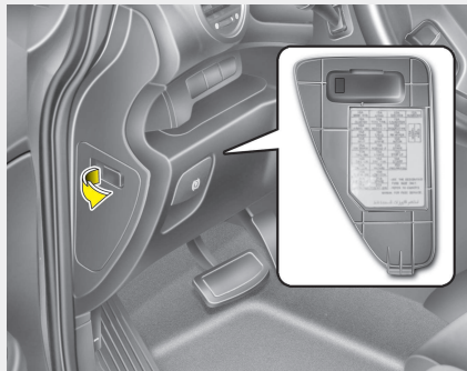
Inner fuse panel
