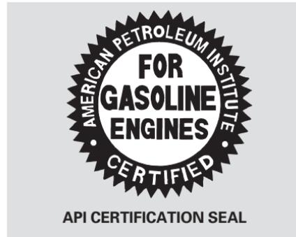
Honda Motor Oil is the preferred 5W-20 lubricant for your vehicle. It is highly recommended that you use Honda Motor Oil in your vehicle for optimum engine protection. Make sure the API Certification Seal says "For Gasoline Engines."
