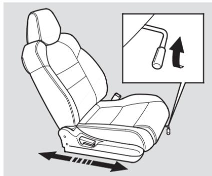
To adjust the seat forward and backward, pull up on the lever under the seat cushion's front edge. Move the seat to the desired position and release the lever. Try to move the seat to make sure it is locked in position.
