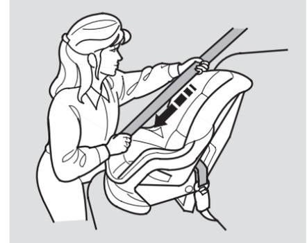
2. To activate the lockable retractor, slowly pull the shoulder part of the belt all the way out until it stops, then let the belt feed back into the retractor.
