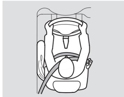
If you ever have a moderate to severe side impact, sensors will detect rapid deceleration and signal the control unit to instantly inflate either the driver’s or the passenger’s side airbag.
