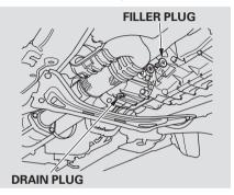
Check the fluid in the transfer assembly with the vehicle sitting on level ground. Remove the filler plug and check that the fluid level is up to the edge of the filler plug hole.
