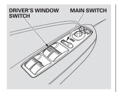
Turn the ignition switch to ON (II) to raise or lower any window. To open the window, push the switch down and hold it. Release the switch when you want the window to stop. Pull back on the switch and hold it to close the window.
