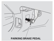
To apply the parking brake, push the pedal down with your foot. To release it, push on the pedal again. The parking brake indicator on the instrument panel should go out when the parking brake is fully released with the engine running (see page 59).
