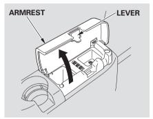
Auxiliary input jacks and headphone connectors for the rear entertainment system are under the third seat armrest on the passenger's side. To access these connectors. open the cover by pulling up on the lever.
