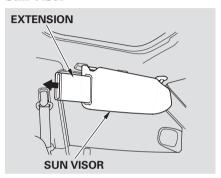
When using the sun visor for the side window, remove the support rod from the clip and swing it out. Slide the extension out to get more coverage on the side window.
