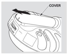
The batteries are under the domed covers on the back of each earpiece. To remove a cover, press down on it with your thumb, slide it backward (away from the headband), then lift it up. Remove the batteries and note their polarity. Install the new batteries in the earpiece with the same polarity. Set the cover in place, then slide it up until it locks. Each headphone uses two AAA batteries.
