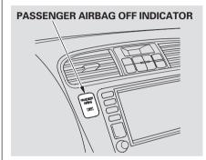
This indicator alerts you that the passenger's front airbag has been shut off. It does not mean there is a problem with the airbag.
