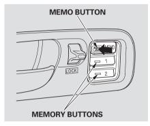
3. Press and release the MEMO button on the control panel. You will hear a beep. Immediately press and hold one of the memory buttons (1 or 2) until you hear two beeps. The indicator in the memory button will come on. The current positions of the driver's seat and outside mirrors are now stored.
