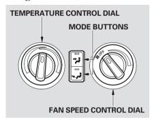
Press the RR A/C MANUAL button to enable the rear A/C control panel. The light in the button will come on. A passenger in the second row can then use the temperature control dial, fan speed dial, and mode buttons to adjust the temperature and airflow to their preference. This is limited by the system's minimum and maximum temperature.
