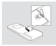
The remote control uses two AA batteries. To replace the batteries, put a coin in the notch on the back. Turn it one-quarter, then slide the cover off. Remove the old batteries. Make sure the polarity of the new batteries is correct when you install them. Slide the cover on until it locks.
