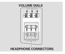
There are three headphone connectors for the third seat passengers. Each connector has its own volume control. These handphones are not supplied with the vehicle
