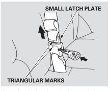
To unlatch the detachable anchor, insert a key into the slot on the side of the small buckle. Line up the triangle marks on the plate and buckle when reattaching the belt and buckle.
