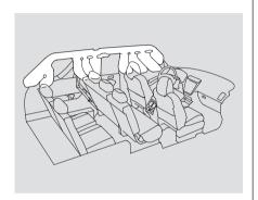
Your vehicle also has side curtain airbags to help protect the heads of the driver, front passenger, and passengers in the outer rear seating positions during a moderate to severe side impact or rollover.
