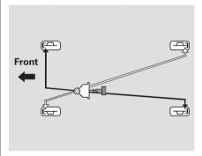
The hydraulic system that operates the brakes has two separate circuits. Each circuit works diagonally across the vehicle (the left-front brake is connected with the right-rear brake, etc.). If one circuit should develop a problem, you will still have braking at two wheels.
