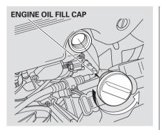
Unscrew and remove the engine oil fill cap on top of the valve cover. Pour in the oil slowly and carefully so you do not spill. Clean up any spills immediately. Spilled oil could damage components in the engine compartment. Install the engine oil fill cap and tighten it securely. Wait a few minutes and recheck the oil level (see page 161). Do not fill above the upper mark on the dipstick; you could damage the engine.
