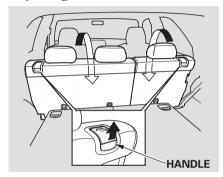
To change the seat-back angle of the seats in the second row, pull up on the handle on the outside of the seat-back.
