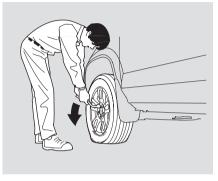
11.Loosen each wheel nut 1/2 turn with the wheel wrench.
