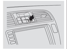
The rear window defogger will clear fog, frost, and thin ice from the window. Push the defogger button to turn it on and off. The indicator in the button lights to show the defogger is on. If you do not turn it off, the defogger will shut itself off after about 15 minutes. It also shuts off when you turn off the ignition. You have to turn it on again when you restart the vehicle.
