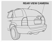
Whenever you shift to R (Reverse) with the ignition switch in the ON (II) position, the rear view is shown in the navigation system display.
