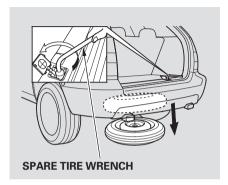
8. Put the wheel nut wrench on the hoist shaft. Turn the wrench counterclockwise to lower the spare tire to the ground.
