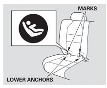
Your vehicle is equipped with LATCH (Lower Anchors and Tethers for Children) at the outer second row seats. The lower anchors are located between the seat-back and seat bottom, and are to be used only with a child seat designed for use with LATCH.
