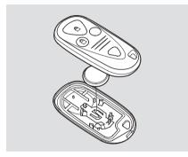
To replace the battery, place a cloth on the edge of the transmitter and remove the upper half by carefully prying on the edge with a small flattip screwdriver. Remove the old battery and insert a new battery with the + side facing up. Snap the two halves of the transmitter case back together.
