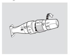
The automatic wiper system senses rainfall and automatically turns on the windshield wipers. To enable sensing, turn the rotary switch at the end of the wiper lever to AUTO.
