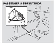
To open the passenger's side, pull the right edge of the cover.
