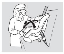
5. Push and pull the child seat forward and from side to side to verify that it is firmly secured. If the child seat is not secure, unlatch the belt, allow it to retract fully, then repeat these steps.
