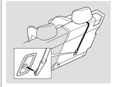
5. Route the tether strap through the legs of the head restraint, then attach the hook to the anchorage point on the back of the seat back.
