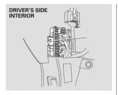
The vehicle's fuses are located in five fuse boxes.
