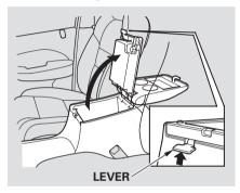
Your vehicle is equipped with a flipover center console lid that provides a tray and a beverage holder for the second row passengers. To open the beverage holders, pull up the center lever on the center console and lift the lid.
