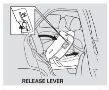
To get into the third row seats, pull up the lever on the side of the passenger's side second row seatback. The seat-back will tilt forward, and the seat will slide forward.
