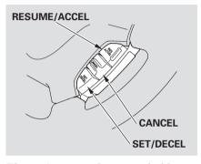
The cruise control may not hold the set speed when you are going up and down hills. If your speed increases going down a hill, use the brakes to slow down. This will cancel the cruise control. To resume the set speed, press the RESUME/ACCEL button. The indicator on the instrument panel will come back on.
