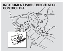
The dial on the instrument panel controls the brightness of the instrument panel lights. Turn the dial to adjust the brightness.
