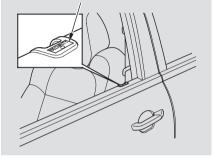
Once the security system is set, opening any door or the tailgate without using the key or the remote transmitter, or the hood, will cause it to alarm. It also alarms if the radio, navigation and DVD components are removed from the dashboard or the wiring is cut.
