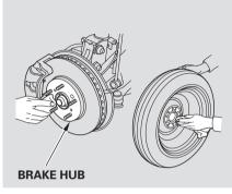
15.Before mounting the spare tire, wipe any dirt off the mounting surface of the wheel and hub with a clean cloth. Wipe the hub carefully; it may be hot from driving.
