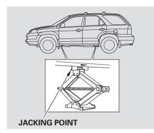
12. Place the jack under the jacking point nearest the tire you need to change. It is pointed to by a  $\triangle$ mark molded into the underside of the body. Turn the end bracket clockwise until the top of the jack contacts the jacking point. Make sure the jacking point tab is resting in the jack notch.
