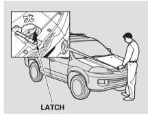
2. Put your fingers under the front edge of the hood to the left of center. Slide your hand to the left until vou feel the hood latch handle. Push this handle up until it releases the hood. Lift the hood.
