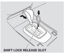
To release the reverse lockout, move the shift lever from Neutral to Reverse, then to Park.
