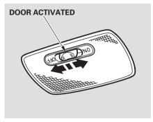
The cargo area light has a threeposition switch. In the OFF position, the light does not come on. In the center position, it comes on when you open the tailgate or doors. In the ON position, it stays on continuously.
