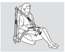
For added protection, the front seat belts are equipped with automatic seat belt tensioners. When activated, the tensioners immediately tighten the belts to help hold the driver and a front passenger in place. The tensioners are designed to activate in any collision severe enough to cause a front, side, or side curtain airbag to inflate.
