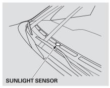
The climate control system has two sensors. A sunlight sensor is in the top of the dashboard, and a temperature sensor is next to the steering column. Do not cover the sensors or spill any liquid on them.
