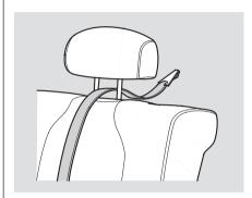
1. After securing the child seat in the desired position (see page 44), route the tether strap over the top of the seat-back and between the head restraint legs.
