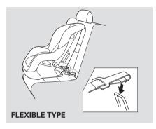
Other LATCH-compatible seats have a flexible-type connection as shown above.
