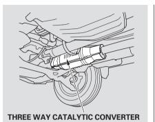
A defective three way catalytic converter contributes to air pollution, and can impair your engine's performance. Follow these guidelines to protect your vehicle's three way
