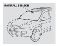
The rainfall sensor is located in the windshield near the rearview mirror. If the sensor is covered with mud, oil, dust, etc., the wipers may not operate properly or may operate unexpectedly.
