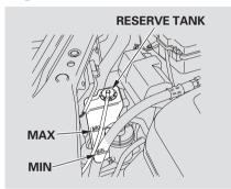
Look at the coolant level in the radiator reserve tank. Make sure it is between the MAX and MIN lines. If it is below the MIN line, see Adding **Engine Coolant** on page 208 for information on adding the proper coolant
