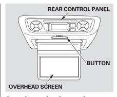
Open the overhead screen by pushing on the button. The screen will swing down part-way. Pivot the screen the rest of the way. If you pivot the screen too far forward, past the detent, the display will turn off. Pivot the screen back to the detent to turn the display back on. To close the screen, pivot it up until it latches.
