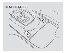
Both front seats are equipped with seat heaters. The ignition switch must be in the ON (II) position to use them. Push the front of the switch, HI, to rapidly heat up the seat. After the seat reaches a comfortable temperature, select LO by pushing the back of the switch. This will keep the seat warm.
