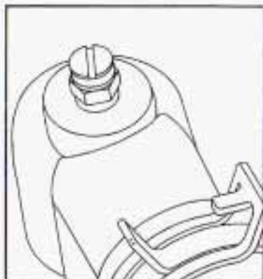
3400 V6 BLEED VALVE #1
