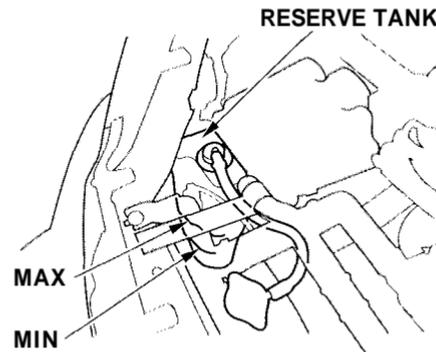
Look at the coolant level in the radiator reserve tank. Make sure it is between the MAX and MIN lines. If it is below the MIN line, see **Adding Engine Coolant** on page [201](#) for information on adding the proper coolant.
