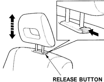
The head restraints adjust for height. You need both hands to adjust the restraint. Do not attempt to adjust it while driving. To raise it, pull upward. To lower the restraint, push the release button sideways and push the restraint down.
