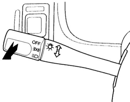
To change between low beams and high beams, pull the turn signal lever until you hear a click, then let go. The blue high beam indicator will light (see page 55).
