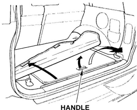
To remove the table, pull up the carpet. Lift and pull on the handle to slide the table out.
