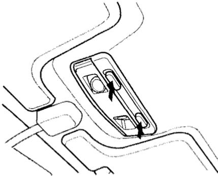
Turn on the spotlight by pushing the button next to each light. Push the button again to turn it off. You can use the spotlights at all times.
