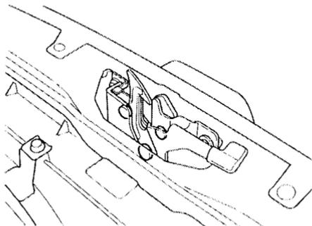
Clean the hood latch assembly with a mild cleaner, then lubricate it with a multipurpose grease. Lubricate all the moving parts, including the pivot. Follow the time and distance recommendations in the Maintenance Schedule. If you are not sure how to clean and grease the latch, contact your Honda dealer.
