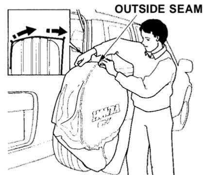
25. Starting at the top of the tire, position the outside seam of the cover slightly over the outside edge of the tire. Pull the cover on, a little at a time, and alternate side to side along the tire until you reach the bottom.
