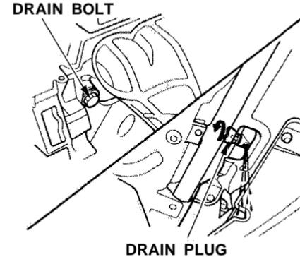
4. Loosen the drain plug on the bottom of the radiator. The coolant will drain through the splash guard. Remove the drain bolt and washer from the engine block.
