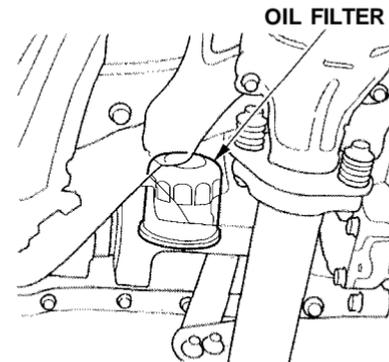
3. Remove the oil filter and let the remaining oil drain. A special wrench (available from your Honda dealer) is required to remove the filter.
