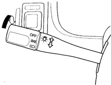
The rotating switch on the left lever controls the lights. Turning this switch to the “☀️” position turns on the parking lights, taillights, instrument panel lights, side-marker lights, and rear license plate lights. Turning the switch to the “☀️” position turns on the headlights.
