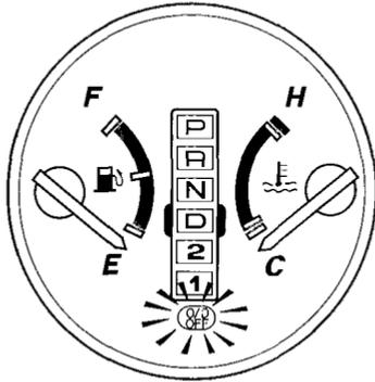
When the Over-Drive is off the transmission selects only the first three gears, but not the fourth. Turn the O/D off to provide engine braking when going down a steep hill. You can also avoid the transmission from cycling between third and fourth gears in stop-and-go driving.
