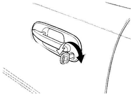
The front doors can be locked and unlocked from the outside with the key.
