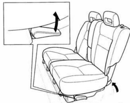
3. Pull up the lever on the side of the rear seat. Lift the rear edge of the seat bottom until the seat latches.
