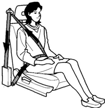
Your Honda has automatic seat belt tensioners for added protection during a moderate to severe frontal collision.
