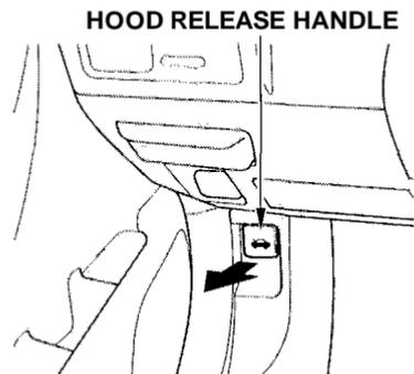
1. Shift to Park or Neutral and set the parking brake. Pull the hood release handle located under the lower left corner of the dashboard. The hood will pop up slightly.
