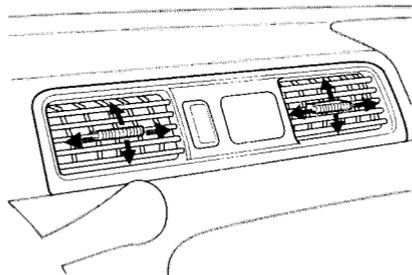
You can adjust the direction of the air coming from the dashboard vents by moving the tab in the center of each vent up-and-down and side-to-side.
