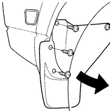
1. The rear side marker light assembly is behind the rear wheel. You can reach the light assembly from the rear wheel housing.
