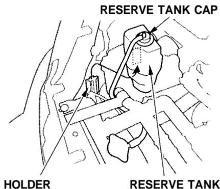
5. Remove the reserve tank from its holder by pulling it straight up. Drain the coolant, then put the tank back in its holder.
