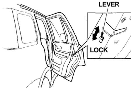
The childproof door locks are designed to prevent children seated in the rear from accidentally opening the rear doors. Each rear door has a lock lever near the edge. With the lever in the LOCK position, the door cannot be opened from the inside regardless of the position of the lock tab. To open the door, pull the lock tab up and use the outside door handle.
