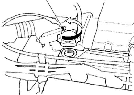
To add oil, unscrew and remove the engine oil fill cap on top of the valve cover. Pour in the oil, and install the engine oil fill cap. Tighten it securely. Wait a few minutes and recheck the oil level. Do not fill above the upper mark; you could damage the engine.
