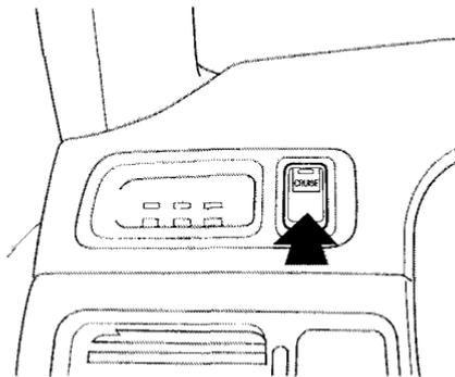
1. Push in the Cruise Control Master Switch to the left of the steering column. The indicator in the switch will light.
