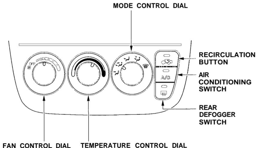
These settings direct all the air flow to the defroster vents at the base of the windshield and the side window defroster vents. The air flow will get warmer and clear the windows faster as the engine warms up. You can close the side vents with the dial beside each vent. This will send more warm air to the windshield defroster vents.
