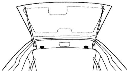
Your Honda has two attachment points for securing a tether-style child seat to the vehicle.
