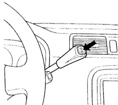
The Over-Drive (O/D) is on whenever you turn the ignition ON (II). You can turn it off by pressing the O/D switch on the edge of the shift lever. The O/D OFF indicator on the instrument panel next to the shift lever position indicator will come on.
