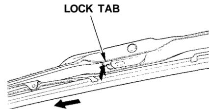
2. Disconnect the blade assembly from the wiper arm by pushing in the lock tab. Hold it in while you push the blade assembly toward the base of the arm.
