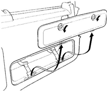
To use the tailgate pocket, turn the knobs and remove the lid. Items stored in this pocket can be secured by the belts inside the pocket.
