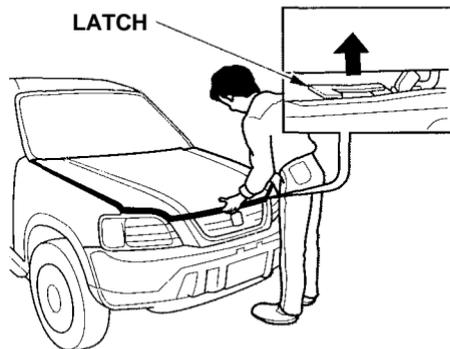
2. Standing in front of the vehicle, put your fingers under the front edge of the hood to the right of center. Slide your hand to the left until you feel the hood latch handle. Push this handle up until it releases the hood. Lift the hood.
