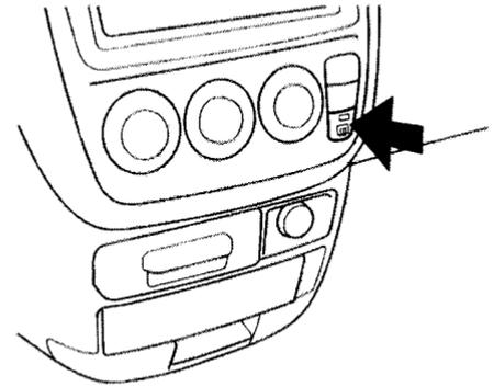
The rear window defogger will clear fog, frost, and thin ice from the window. Push the defogger button to turn it on and off. The light in the button lights to show the defogger is on. If you do not turn it off, the defogger will shut itself off after about 25 minutes. It also shuts off when you turn off the ignition. You have to turn it on again when you restart the vehicle.
