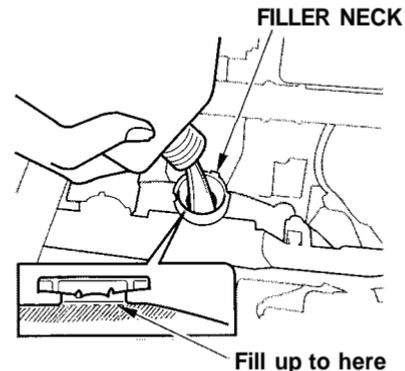
8. Pour coolant into the radiator up to the base of the filler neck.
