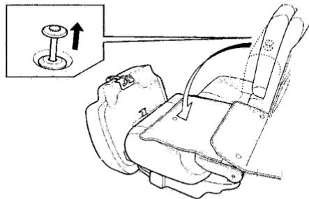
3. Remove the head restraint and pull up on the knob on the top of the seat-back. Pivot the seat-back forward.
