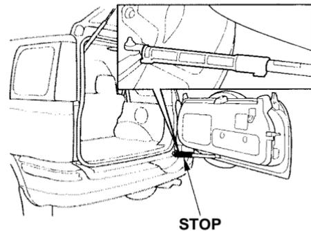
To keep the tailgate door open on an incline, use the stop in the tool kit. The tool kit is in the right cargo floor pocket. Put the stop on the support strut as shown.
