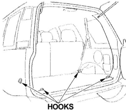
The hooks on the floor of the cargo area enable you to tie down items stored in the back. Make sure all stored items are secured before driving.
