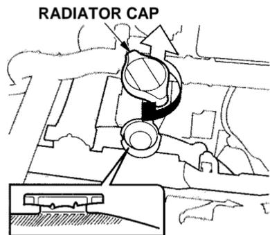
2. Turn the radiator cap counter-clockwise, without pressing down on it, until it stops. This relieves any pressure remaining in the cooling system.
