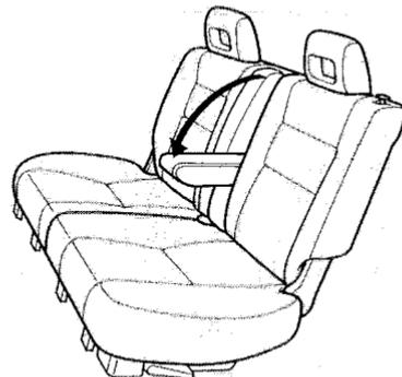
The rear seat armrest is located at the center of the rear seat. Pivot it down to use it.
