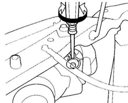
6. Check the vertical angle gauge. The bubble should be centered underneath the longest scribe mark on the gauge.
