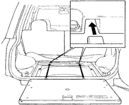
Put the projections on the table into the holes in the cargo area floor.
