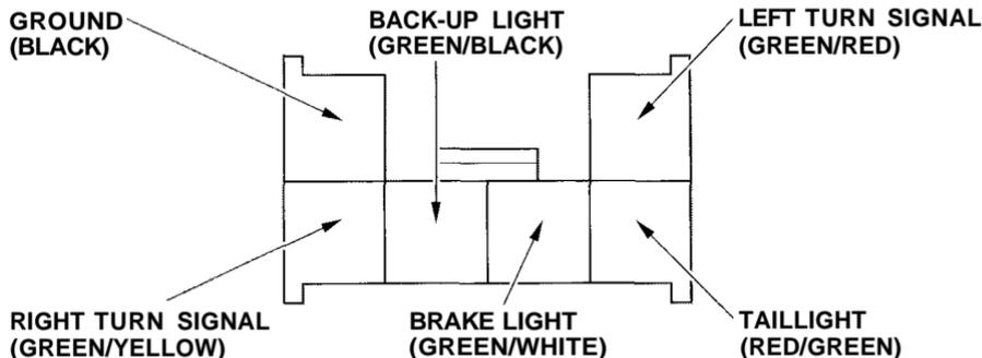
Your vehicle has a trailer lighting connector located behind the left side panel in the cargo area. Refer to the drawing above for the wiring color code and purpose of each pin.
