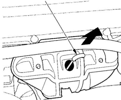
Check the engine oil level every time you fill the vehicle with fuel. Wait a few minutes after turning the engine off before you check the oil.
