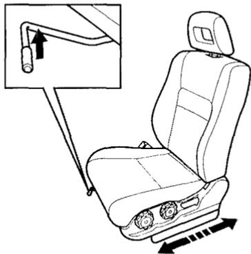
To adjust the seat forward and backward, pull up on the lever under the seat cushion's front edge. Move the seat to the desired position and release the lever. Try to move the seat to make sure it is locked in position.
