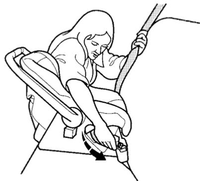
1. With the child seat in the desired back seating position, route the belt through the child seat according to the seat maker's instructions, then insert the latch plate into the buckle.
