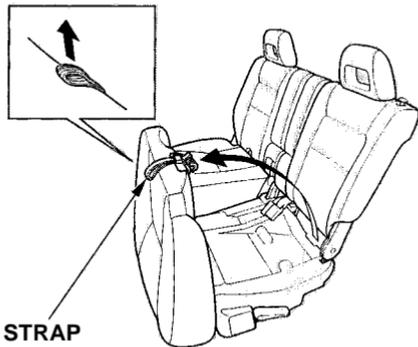
2. Pull the strap to release the seat bottom. Pivot the seat bottom forward.
