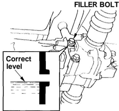
Check the fluid level with the rear differential at normal operating temperature and the vehicle sitting on level ground. Remove the differential fluid filler bolt and washer and carefully feel inside the bolt hole with your finger. The fluid level should be up to the edge of the bolt hole. If it is not, slowly add Genuine Honda Dual Pump Fluid until it starts to run out of the hole. Reinstall the filler bolt and tighten it
