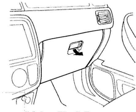
Open the glove box by pulling the bottom of the handle. Close it with a firm push. Lock or unlock the glove box with the master key.
