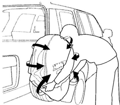
8. Pull out the cover's two lower flaps. Don't pull the top of the cover, or you will tear it.
