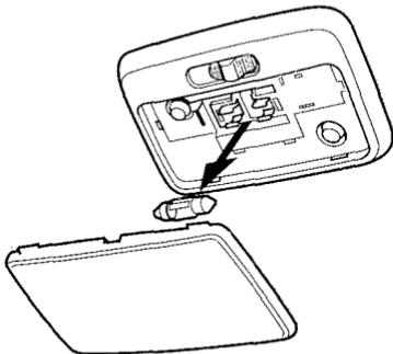
1. Remove the lens by carefully prying on the edge of the lens with a fingernail file or a small flat-tip screwdriver. Do not pry on the edge of the housing around the lens.
