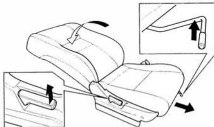
2. Lift the slide lever and slide the front seat forward as far as it will go. Pull up the seat-back angle adjustment lever, then pivot the seat-back backward. Release the lever when the seat-back is even with the cushion on the rear seat.
