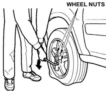
13. Loosen the five wheel nuts 1/2 turn with the wheel wrench.
