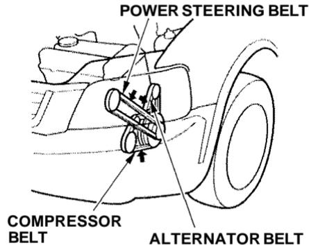
Check the condition of the three drive belts. Examine the edges of each belt for cracks or fraying. Check the tension of each belt by pushing on it with your thumb midway between the pulleys.
