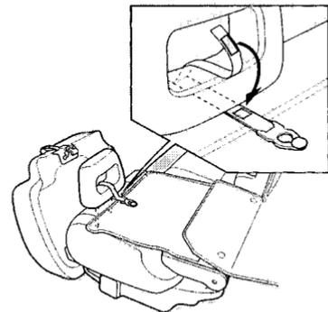
Put the head restraint behind the seat bottom as shown. Pass the fastening strap through the hole of the head restraint and fasten it with the velcro strap.
