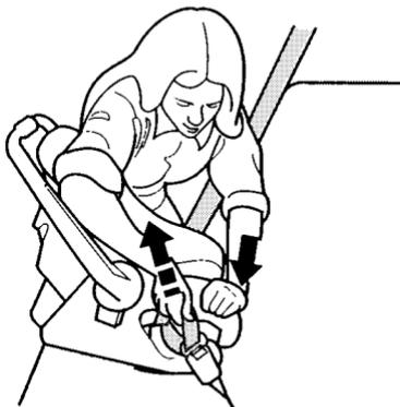
4. After confirming that the belt is locked, grab the shoulder part of the belt near the buckle and pull up to remove any slack from the lap part of the belt. Remember, if the lap part of the belt is not tight, the child seat will not be secure. To remove slack, it may help to put weight, on the child seat, or push on the back of the seat, while pulling up on the belt.
