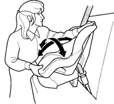
5. Push and pull the child seat forward and from side to side to verify that it is secure enough to stay upright during normal driving maneuvers. If the child seat is not secure, unlatch the belt, allow it to retract fully, then repeat these steps.
