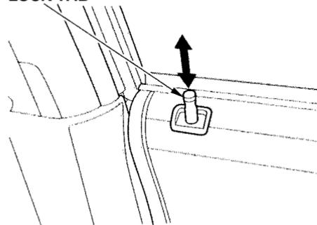
Each door has a lock tab on the top. Push the tab down to lock the door and pull it up to unlock.
