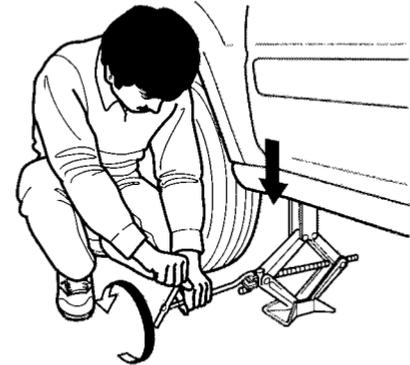
19. Lower the vehicle to the ground and remove the jack.
