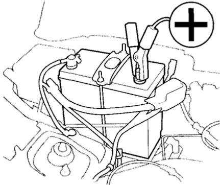
3. Connect one jumper cable to the positive (+) terminal on the booster battery. Connect the other end to the positive (+) terminal on your Honda's battery.
