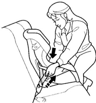
To install a forward-facing child seat in the center back seat with the lap belt, follow instruction number 1 on page 34 for routing and latching the seat belt. Then pull hard on the loose end of the belt to remove any slack; it may help to put weight on the child seat while pulling on the belt. Finally, follow instruction number 5 on page 35 to verify that the child seat is secure.
