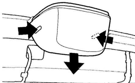
1. Remove the light assembly cover by pushing the tabs on both sides and pulling the cover down.
