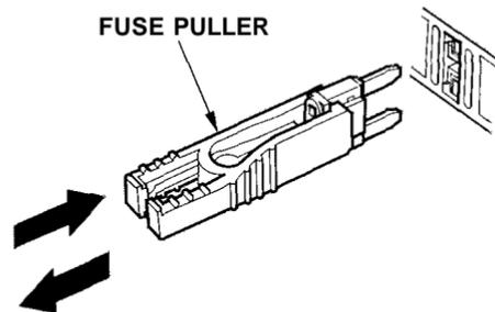
4. Check the smaller fuses in the under-hood fuse box and all the fuses in the interior fuse box by pulling out each fuse with the fuse puller provided in the door of the interior fuse box.
