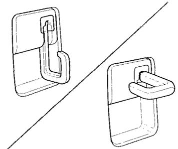
The hook on the tailgate door pivots, allowing items to be stored in different ways. Make sure any items put on this hook weigh less than 6.5 lbs (3 kg), or you could damage the hook.
