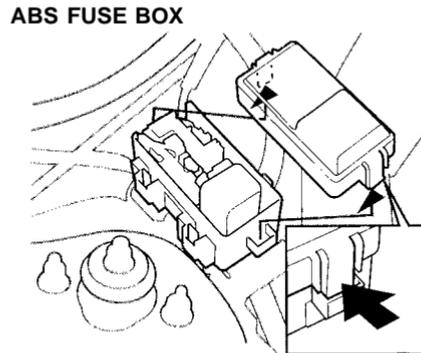
Vehicles equipped with ABS have a third fuse box for the ABS. It is in the engine compartment on the passenger's side.
