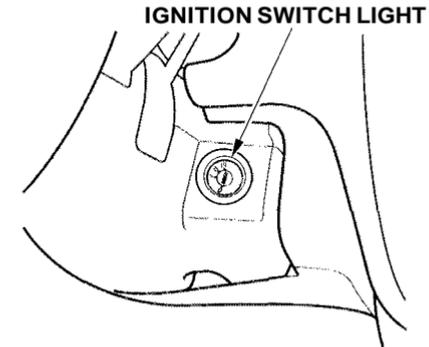
The ignition switch light comes on when you open the driver's door, and stays on several seconds after you close the door.
