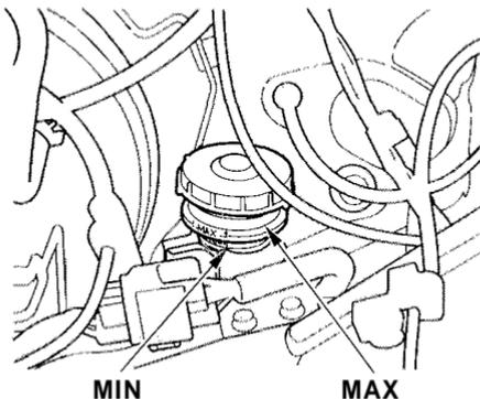
The fluid should be between the MIN and MAX marks on the side of the reservoir. If it is not, add brake fluid to bring it up to that level. Use the same fluid specified for the brake system.
