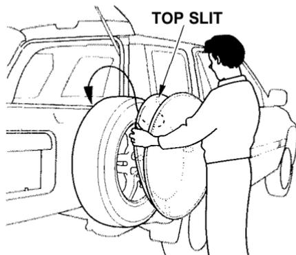
23. Hold the cover at the 10 o'clock and 2 o'clock positions, then place the top of it over the spare tire, making sure the top slit on the back of the cover is vertical.
