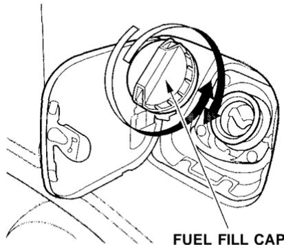
3. Remove the fuel fill cap slowly. You may hear a hissing sound as pressure inside the tank escapes.
