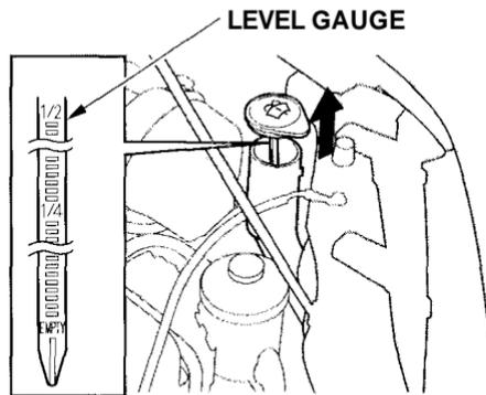
The windshield washer reservoir is located behind the driver's side headlight. Check the reservoir's fluid level by removing the cap and looking at the level gauge attached to the cap.
