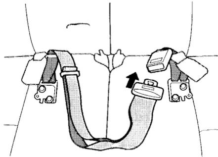
To fasten the belt, insert the latch plate into the buckle marked **CENTER**, then tug on the belt to make sure the buckle is latched.
