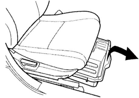
A storage box is located under the front passenger's seat. To use it, pull upward slightly on the front center edge of the box to disengage the locking tabs then pull forward to slide the box out.
