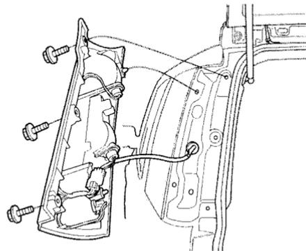
1. Open the tailgate. Remove the three screws and remove the rear light assembly from the rear pillar.
