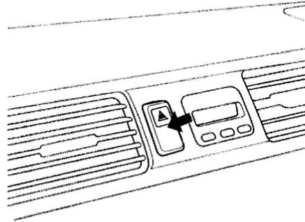
Push the red button between the center air vents to turn on the hazard warning lights (four-way flashers). This causes all four outside turn signals and both indicators in the instrument panel to flash. Use the hazard warning lights if you need to park in a dangerous area near heavy traffic, or if your vehicle is disabled.
