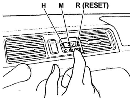
The digital clock displays the time with the ignition switch ON (II).
