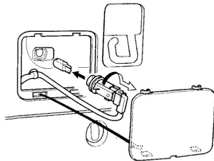
1. Remove the cover by carefully prying on the edge of the cover in the middle with a small flat-tip screwdriver.
