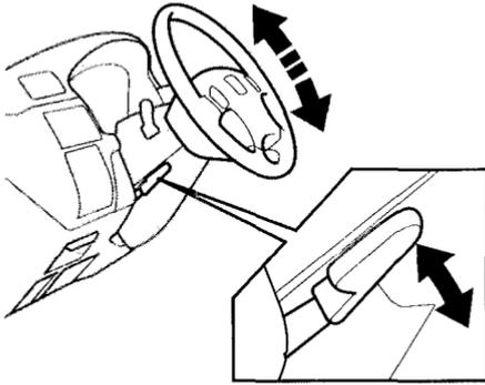
To adjust the steering wheel upward or downward:
