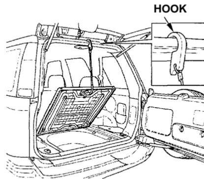
3. Pull up the cargo area carpet and open the cargo area floor. To keep the cargo area floor out of the way, attach the hook to the tailgate sill as shown.
