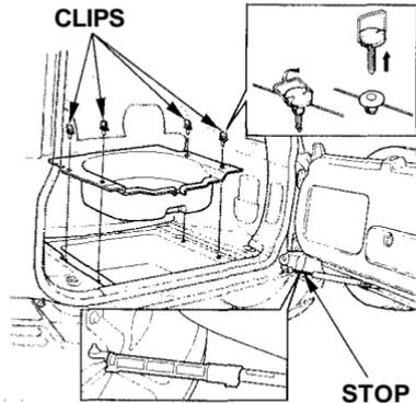
5. The jack is under the cargo storage bin. Remove each of the four clips holding the bin by pulling straight up on the ring. Remove the bin.
