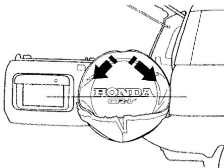
24. Step back to check the alignment of the logo. If needed, move the cover left or right until the logo is straight.
