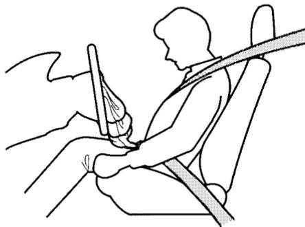
After inflating, the airbags immediately deflate, so they won't interfere with the driver's visibility, or the ability to steer or operate other controls.
