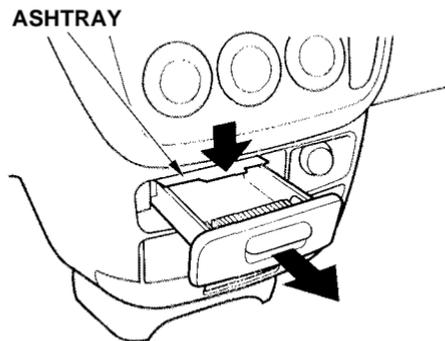
Open the front ashtray by pulling on the bottom edge. Push it in to close it. To remove the ashtray for emptying, push down on the metal plate inside, then pull the ashtray out completely.
