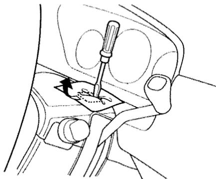
4. Insert the key in the Shift Lock Release slot on the steering column.
