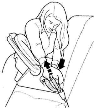
To install a rear-facing child seat in the center back seat with the lap belt, follow instruction number 1 on page 30 for routing and latching the seat belt. Then pull hard on the loose end of the belt to remove any slack (it may help to put weight on the child seat while pulling on the belt). Finally, follow instruction number 5 on page 31 to verify that the child seat is secure.
