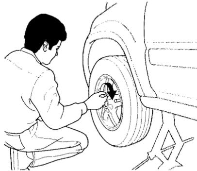
18. Put on the spare tire. Put the wheel nuts back on finger-tight, then tighten them in a crisscross pattern with the wheel wrench until the wheel is firmly against the hub. Do not try to tighten them fully.
