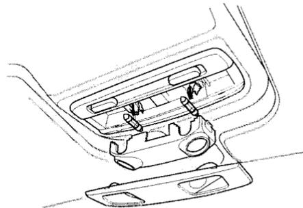
2. Remove the bulb by pulling it straight out of its metal tabs.
