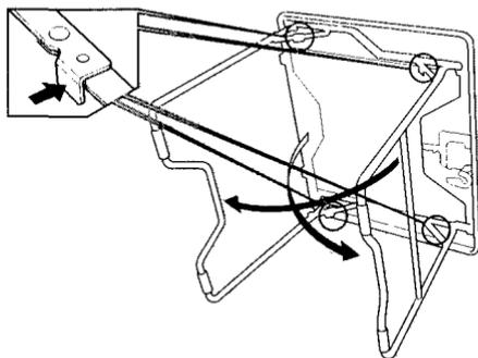
Unfold the legs. Lock them in place by pushing on the middle of the locking arms. Make sure all four are locked.
