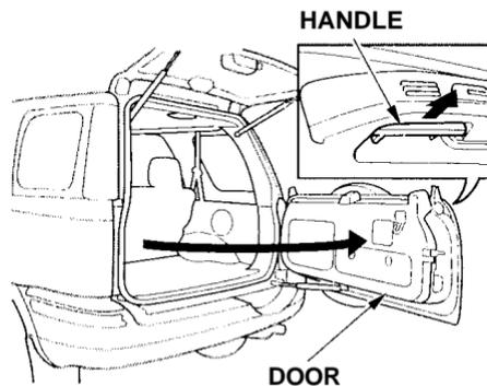
4. Pull the handle on the door and pull the door open.
