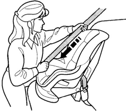
2. To activate the lockable retractor, slowly pull the shoulder part of the belt all the way out until it stops, then let the belt feed back into the retractor (you might hear a clicking noise as the belt retracts).
