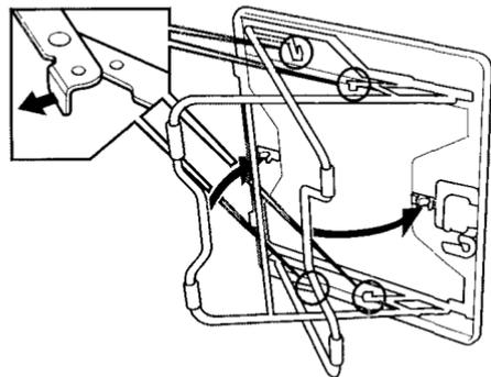
To fold the legs, pull on the middle of each locking arm.
