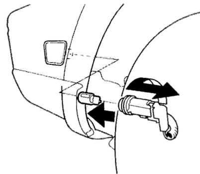
3. Remove the socket from the rear side marker assembly by turning it one-quarter turn counterclockwise.
