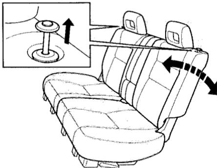
The angle of the rear seat-backs can be adjusted separately. To change the angle of the seat-back, pull up on the knob on the top of the seat-back. Move the seat-back to the desired position, then release the knob. Make sure the seat-back latches in the new position.
