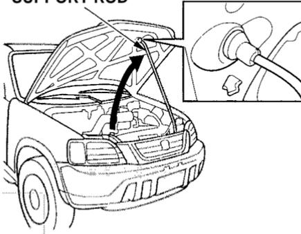
3. Pull the support rod out of its clip and insert the end into the hole on the front of the hood around the center.
