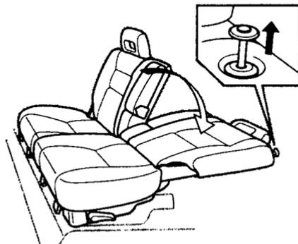
4. Pull up on the knob on top of the seat-back and pivot the rear seat-back backward. Release the knob when the seat-back is reclined as far as it will go.
