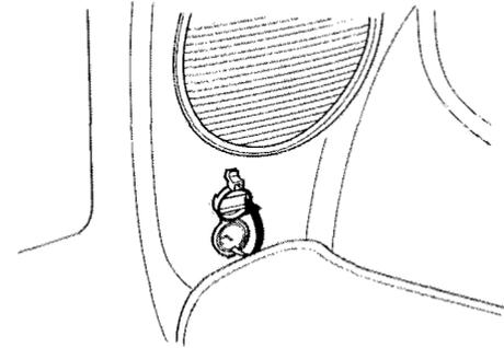
To use the accessory power socket, pull down on the cover. The ignition switch must be in ACCESSORY (I) or ON (II).
