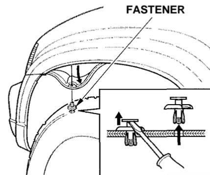
2. Use a flat-tip screwdriver to remove the fastener from the inner fender.
