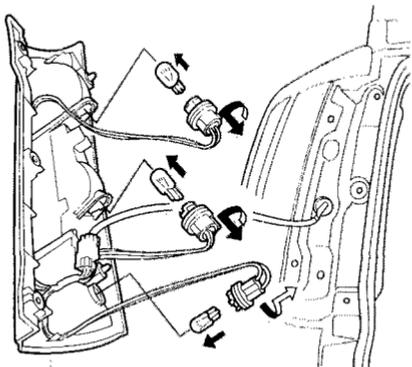
3. Remove the socket by turning it one-quarter turn counterclockwise.
