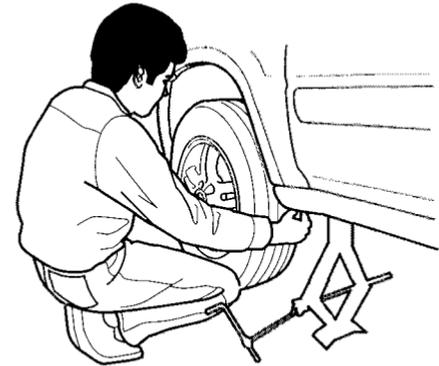
16. Remove the wheel nuts and flat tire. Temporarily place the flat tire on the ground with the outside surface of the wheel facing up. You could scratch the wheel if you put it face down.
