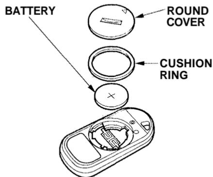
Remove the old battery and note the polarity. Make sure the polarity of the new battery is the same (+ side facing up), then insert it in the transmitter.
