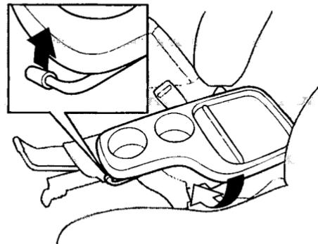
To use the center table, pull up the outside edge of the table until it latches. To store it, pull the lever and lower the table.
