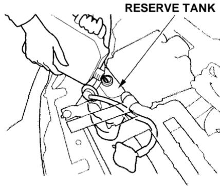
11. Fill the reserve tank to the MAX mark. Install the reserve tank cap.
