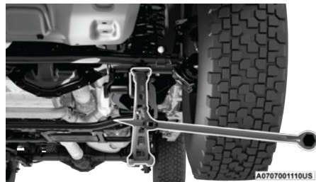
Front Jacking Location
