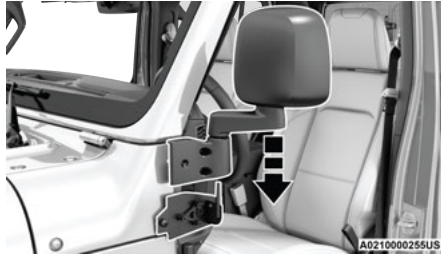
Lower Mirror Assembly Onto Bracket
