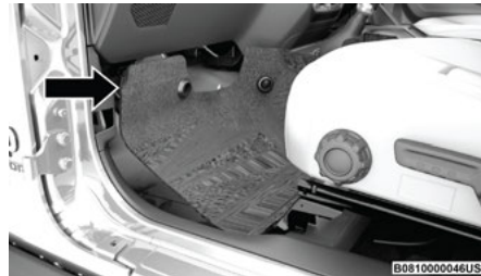
Front Carpet Pulled Away
