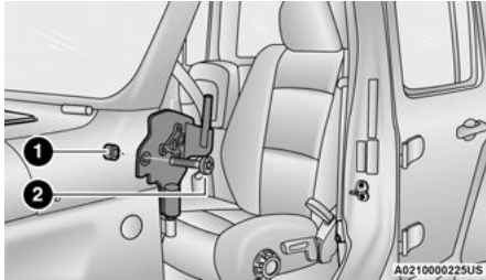
Attaching Mirror Bracket To The Vehicle
