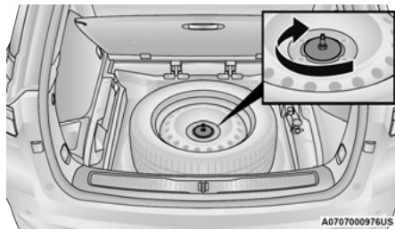
Reinstalling Tire Fastener
