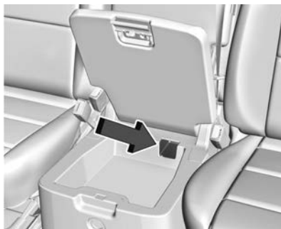
Transmitter Pocket without Bucket Seats (Lower Compartment)
