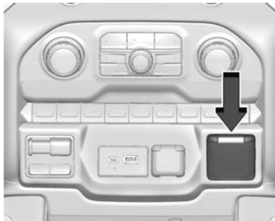
In Cab Power Outlet
