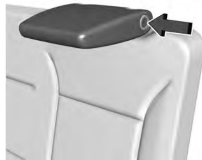
The head restraint will fold forward automatically.
