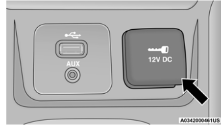
Front Power Outlet
