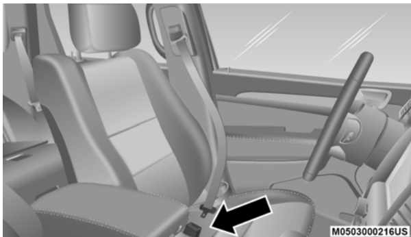
Inserting Latch Plate Into Buckle
