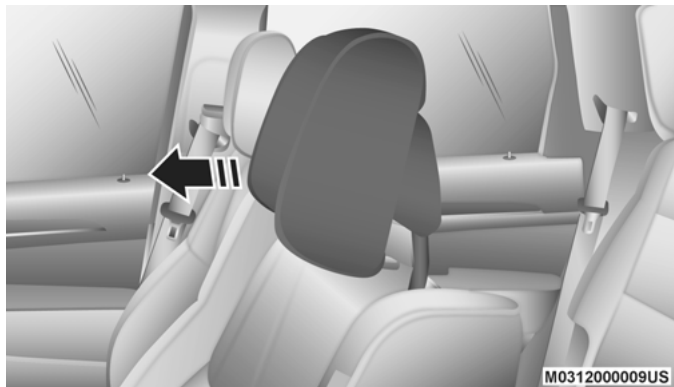
Active Head Restraint (Tilted)
