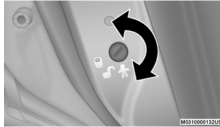
Child-Protection Door Lock Function
