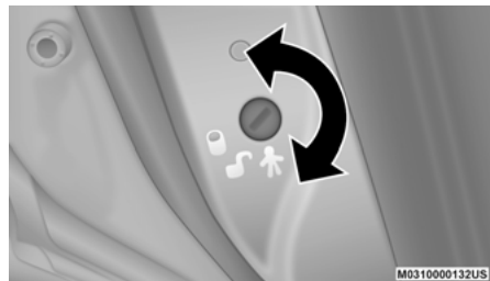
Child-Protection Door Lock Function
