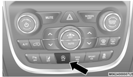
Stop/Start OFF Switch
