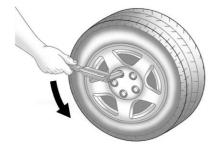
Turn the wheel wrench counterclockwise to loosen all the wheel nuts, but do not remove them yet.
