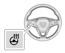
**3** : If equipped with a heated steering wheel, press to turn on or off. A light near the button displays when the feature is turned on.
