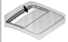
Dirt and debris may collect on the sunroof seal or in the track. This could cause an issue with sunroof operation or noise. It could also plug the water drainage system. Periodically open the sunroof and remove any obstacles or loose debris. Wipe the sunroof seal and roof sealing area using a clean cloth, mild soap, and water. Do not remove grease from the sunroof.
