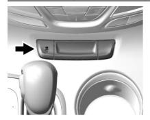
To turn off only TCS, press and release ♣. The traction off light ຝ illuminates in the instrument cluster.
