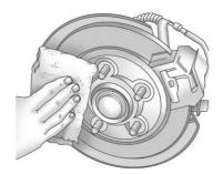
9. Remove any rust or dirt from the wheel bolts, mounting surfaces, and spare wheel.
