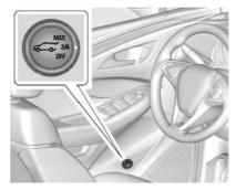
If equipped with a power liftgate, the switch is on the driver door. The vehicle must be in P (Park).
