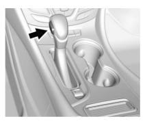
ERS or manual mode allows for the selection of the range of gear positions. Use this mode when driving downhill or to limit the top gear and vehicle speed. The shift position indicator within the Driver Information Center (DIC) will display
