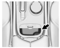
There is a small bin directly in front of the center console. On some models, the bin has a cover. Use the handle to open the covered bin.
