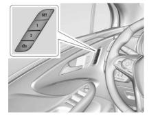
If equipped, memory seats allow two drivers to save and recall their unique seat positions for driving the vehicle, and a shared exit position for getting out of the vehicle. Other feature positions may also be saved, such as power mirrors and power steering wheel, if equipped.
