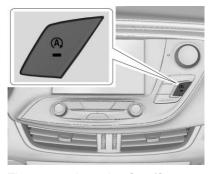
The automatic engine Stop/Start feature can be disabled and enabled by pressing the switch with the A symbol. Auto Stop is enabled each time you start the vehicle.
