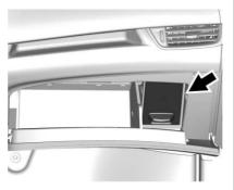
The instrument panel fuse block is in the glove box. To access the fuses, open the fuse panel door from the passenger side by pulling it out.
