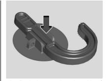
Push down on the other side of the load floor hook to lock into place.
