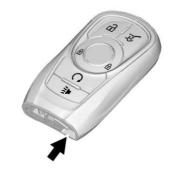
Separate the two halves of the transmitter using a flat tool inserted into the bottom of the transmitter.
