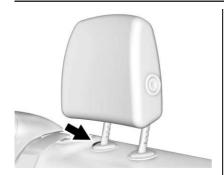
To lower the head restraint, press the button located on the top of the seatback and push the head restraint down. Try to move the head restraint after the button is released to make sure it is locked in place.
