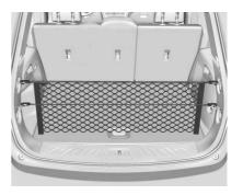
This vehicle may have a convenience net in the rear of the vehicle. Attach it to the cargo tie-downs for storing small loads.
