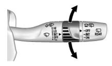
INT: Use for intermittent wipes or Rainsense, if equipped and enabled. To adjust wipe frequency, turn the band up for more frequent wipes or down for less frequent wipes. If Rainsense is enabled, see "Rainsense" later in this section.
