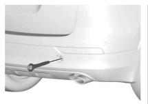
Install the tow eye into the socket and turn it until it is fully tightened.
