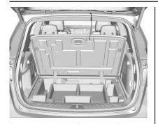
Remove the load floor hook from the holder and hook to the weatherstrip above.
