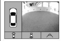
If equipped, a view of the area in front of the vehicle appears in the infotainment display. The front view shows after shifting from R (Reverse) to D (Drive) and when the vehicle is moving forward slower than 8 km/h (5 mph), or when the Park Assist system detects an object within 30 cm (12 in).
