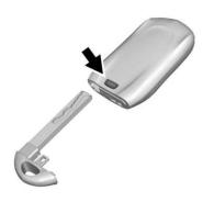
Press the button on the RKE transmitter to remove the key.
