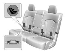
The lower anchors are behind the horizontal openings in the seat cushion trim located below the anchor label.
