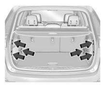
The vehicle may be equipped with six cargo tie-downs in the rear compartment.
