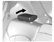
The rear outboard head restraints are designed to be folded. The head restraint can be folded backward to allow for better visibility when the rear seat is unoccupied. To fold the head restraint, press the button on the side of the head restraint.
