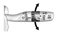
**AUTO:** Move the windshield wiper lever to AUTO. Turn the band on the wiper lever to adjust the sensitivity.
