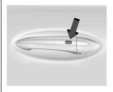
The RKE transmitter must be within 1 m (3 ft) of the liftgate or door being opened. Press the button on the door handle to unlock. See "Keyless Access Operation" in Remote Keyless Entry (RKE) System Operation ▷ 8.
