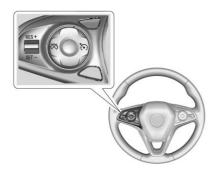
: Press to turn cruise control on or off. A white indicator comes on in the instrument cluster when cruise control is turned on.
