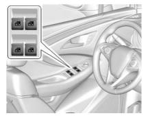
Power windows work when the ignition is on, in ACC/ACCESSORY, or when Retained Accessory Power (RAP) is active. See Retained Accessory Power (RAP) ⇒ 179.
