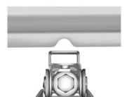
Locate the notch on the sheet metal weld flange. Place the center of the jack lift head on the center of the sheet metal notch.
