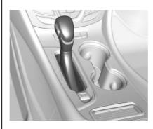
**P**: This position locks the front wheels. Use P (Park) when starting the engine because the vehicle cannot move easily.
