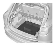
There are no attachments securing the cargo management system. Lift up on both sides to remove the cargo management system.
