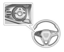
া Press to turn the system on or off. A white cruise control indicator comes on in the instrument cluster.
