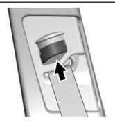
Move the height adjuster up to the desired position by pushing up on the height adjuster.
