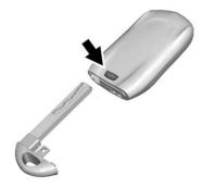
Press the button on the transmitter to access the key.
