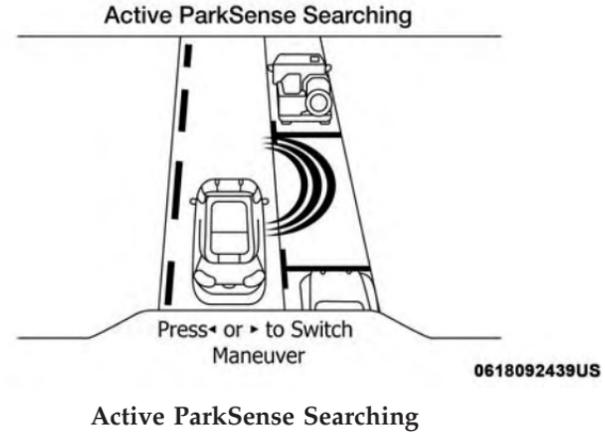
When an available parking space has been found, and the vehicle is not in position, you will be instructed to move forward to position the vehicle for a parallel parking sequence.
