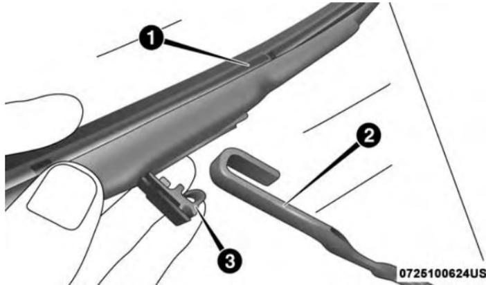
**Wiper Blade Removed From Wiper Arm**
