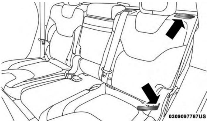
**Rear Sliding Seat Release Lever And Pull Strap**
