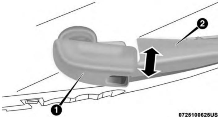
**Wiper Pivot Cap In Unlocked Position**
