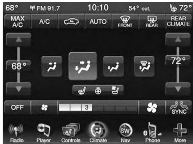
Uconnect 3/3 NAV Automatic Tri-Zone Temperature Controls
