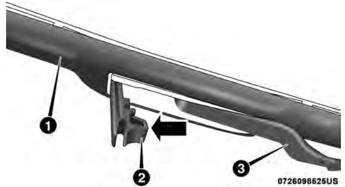
Wiper Blade With Release Tab In Unlocked Position
