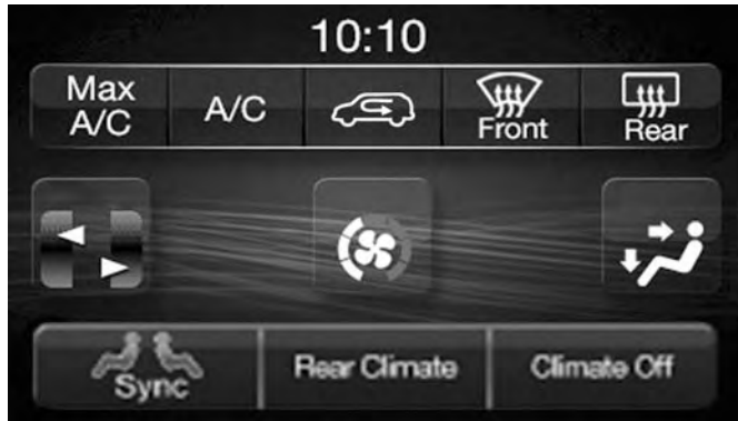
Radio 4.3 Manual 3 Zone Temperature Controls
