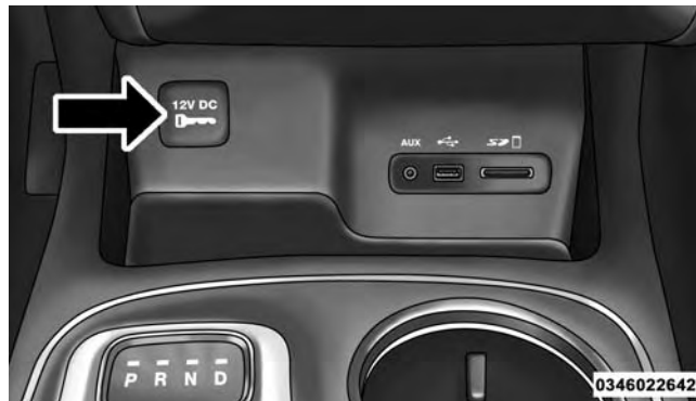
Front Power Outlet
