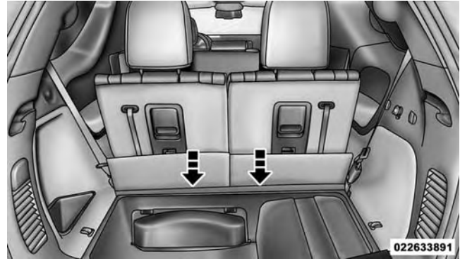
Pulling Down The Carpet Floor Panel To Access Top Tether Strap
