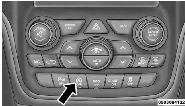
STOP/START Off Switch
