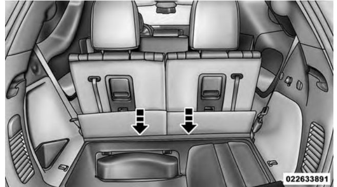
Pulling Down The Carpet Floor Panel To Access Top Tether Strap
