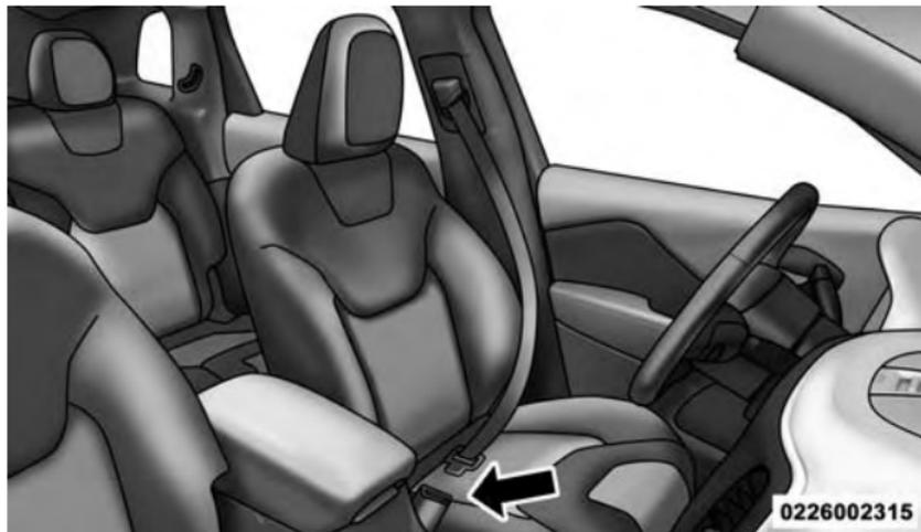
Inserting Latch Plate Into Buckle
