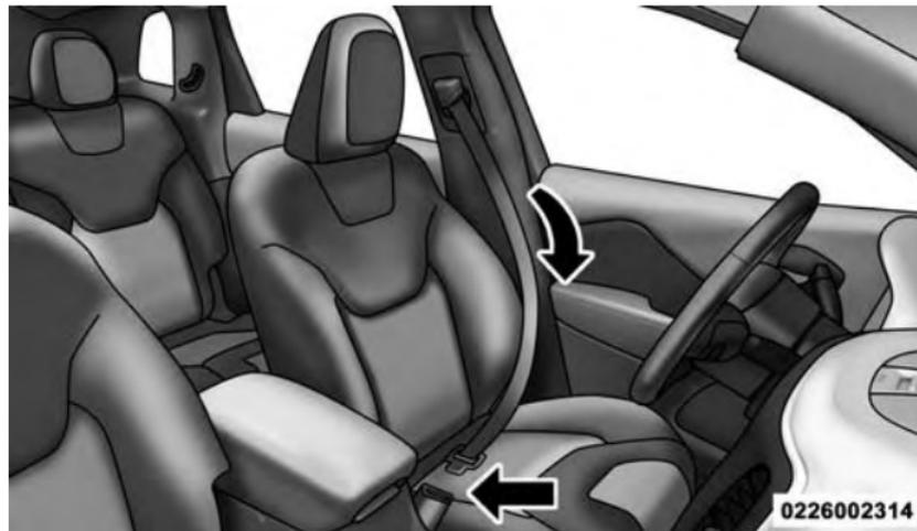
**Pulling Out The Lap/Shoulder Belt Latch Plate**
